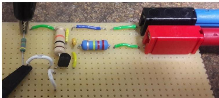
*Figure 31 - Testing 2N3904 bipolar transistor soldered on a stripboard*
