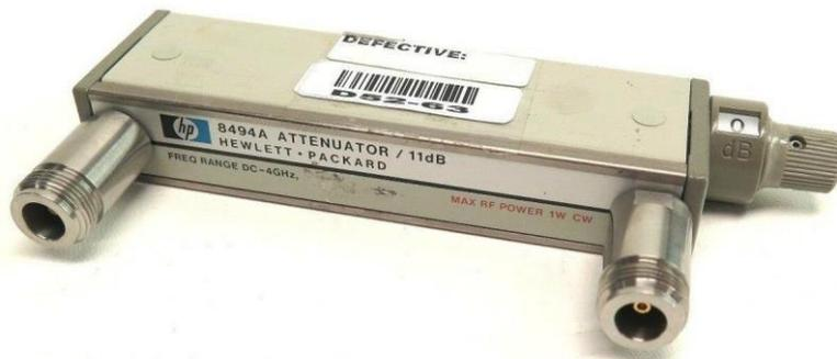
Figure 19 - External attenuator with step adjustment
