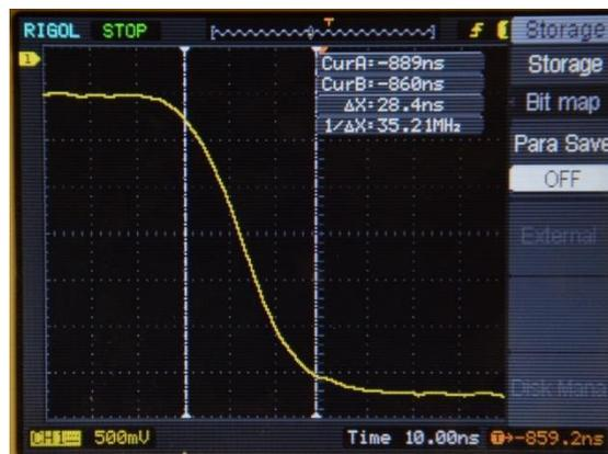
Figure 48 - Switched Capacitance - pulse width determination
