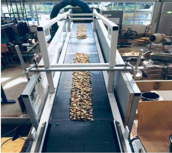
Figure 2.3: (left) Sediment arrangement to check sensor accuracy, (right) sample graphical result, to prove the sensor accuracy
