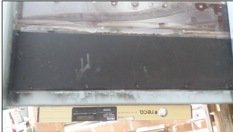
Figure 4.2(a): Digital level at the bottom of flume, to check the required slope
