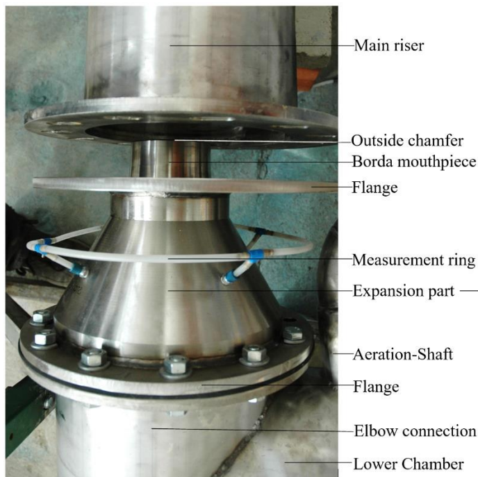
Figure 5-10: Differential orifice throttle small-scale model, (picture: Richter )
