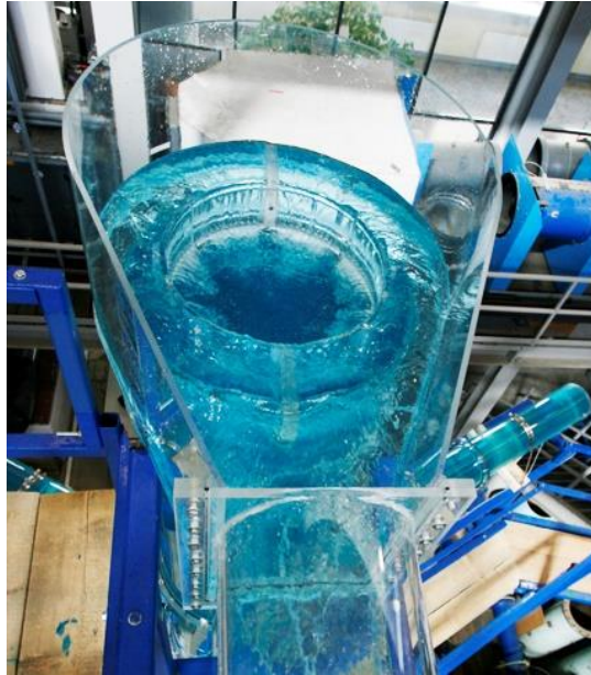
Figure 6-92: Waterfall damping device for Krespa surge tank, time at water column separation ( Richter )
