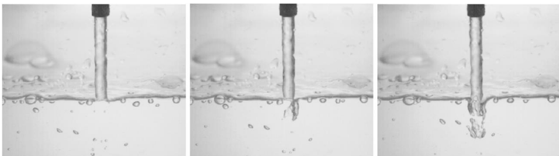
Figure 6-73: Air bubble intrusion mechanism of a single jet ( Danciu [208])
