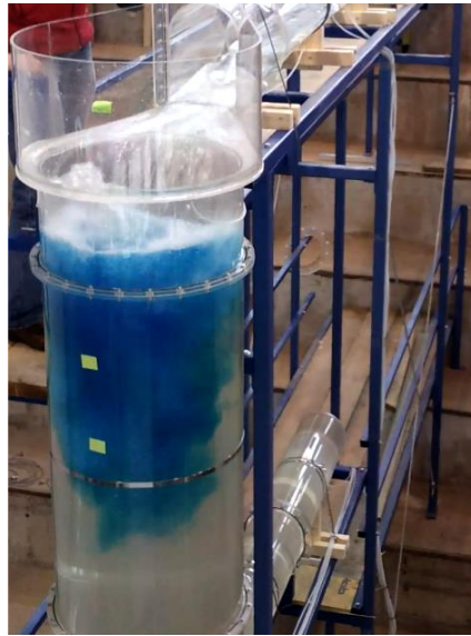
Figure 6-76: Waterfall in physical model test without dampening device ( Richter [43])
