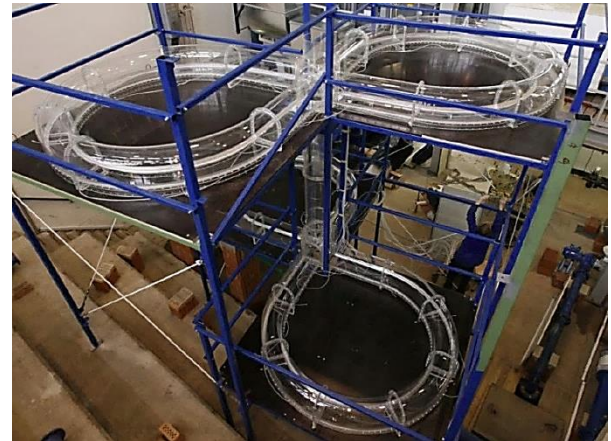
Figure 5-28: Physical model of the surge tank Atdorf in the hydraulic laboratory, (Richter [106])
