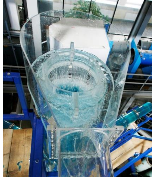
Figure 6-93: Waterfall damping device for Krespa surge tank, transformation of a large waterfall to defined smaller water jets ( Richter )
