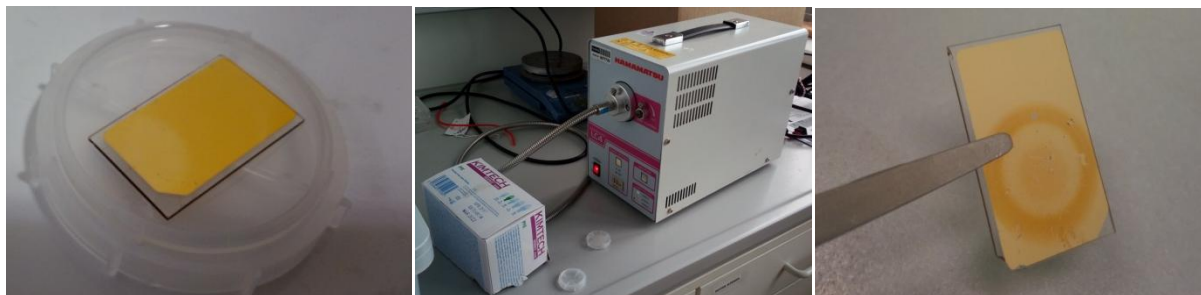
Figure 40: Illumination of lignin and lignin acetate on a gold slide for 20 minutes.
