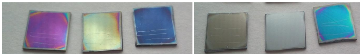
Figure 22: Color variations of AcL thin films directly after the spin coating process.
