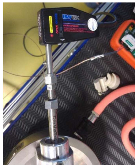
Fig. 5-13: The laser trigger and the ColVisTec Raman probe built in the spectroscopy chamber.
