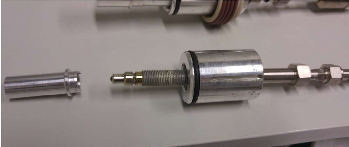
Fig. 5-7: One RPMP with pulled on lid from the spectroscopy chamber. On the left the smaller piston is shown where the probe fits in. Although it is a reflection probe it has a collimator lens to be also prepared for transmission measurements.
