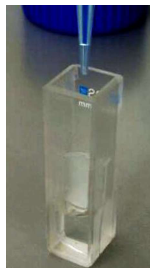
Fig. 5-15: EVA28 strip in a standard cuvette filled up with ethanol.
