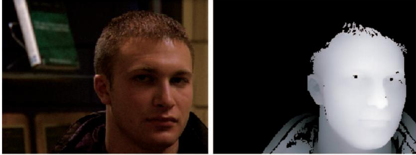
**Figure 2.20:** Aligned 2D and 3D data. Example from FRGC v2.0. Figure taken from [MBO07].
