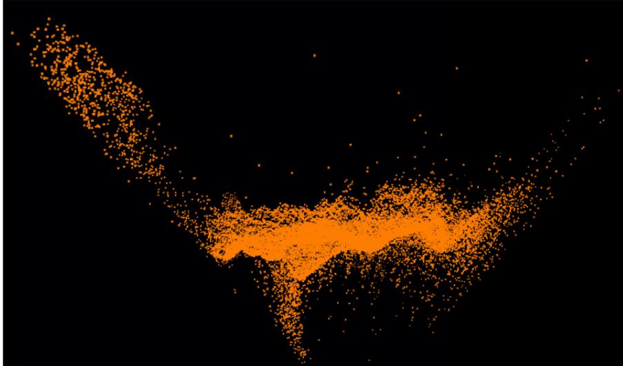
**Figure 3.3:** Exposure time of  $2000 \mu s$ . Face from side view. Good quality of face surface, many outliers (flying pixels) occur around the face.
