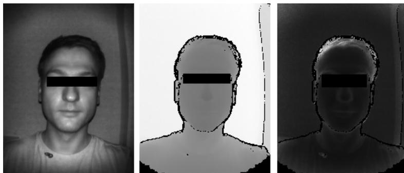
**Figure 2.2:** Example of ToF data, on the left side we illustrate the amplitude data, in the middle the depth data and on the right side a typical noise image. Note that bright pixels in the depth image indicate a higher distance. We observed that the noise data is stronger influenced by reflecting backgrounds than amplitude and depth data.
