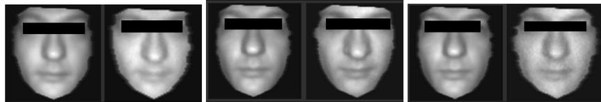
(d) Accepted image in sunlight at a distance of around 50 cm. (e) Accepted image in strong sunlight at a distance of around 30 cm. (f) Accepted image in strong sunlight at a distance of around 50 cm.
