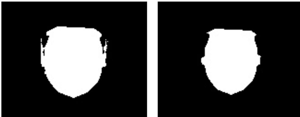
**Figure 4.8:** On the left side, we visualise the coarse binary mask. On the right side, we illustrate the binary mask after the erode operation. The result is a smaller binary mask with less disturbing outliers.
