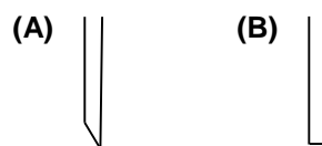
Figure 14: Shape of steel and Teflon cannulas: (A) rigid steel cannula with a sharp tip, (B) flexible Teflon cannula with a blunt end.
