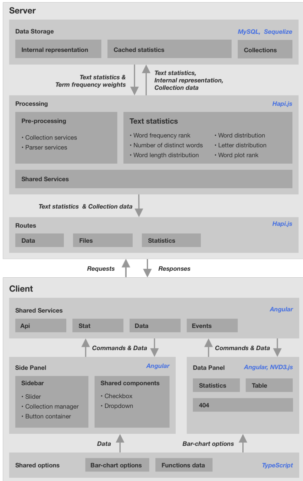
Figure 3.2.: The final architecture of the Infret prototype. Blocks represent component groups. Connections between components are represented with lines between components and represent more than one connection going in one or both directions. The arrows represent the direction of the data flow, while the italic text describes the data transmitted through the connections.
