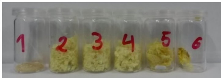
Figure B-4. ATA-47 co-lyophilized with various amount of EB: free enzyme (1), free enzyme lyophilized with PLP (2), 1:0.05 coating (3), 1:0.1 coating (4), 1:0.5 coating (5), and 1:1 coating (6).
