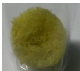
Figure B-5. ATA-47 co-lyophilized with 1:0.5 IL (EB) after the reaction.
