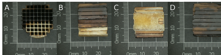
Figure 4.15.: Pictures of the IBIDEN FRAUENTHAL HT ceramics wick after 18 h operation with air as carrier gas. Views: A) front, B) side, C) bottom and D) top
