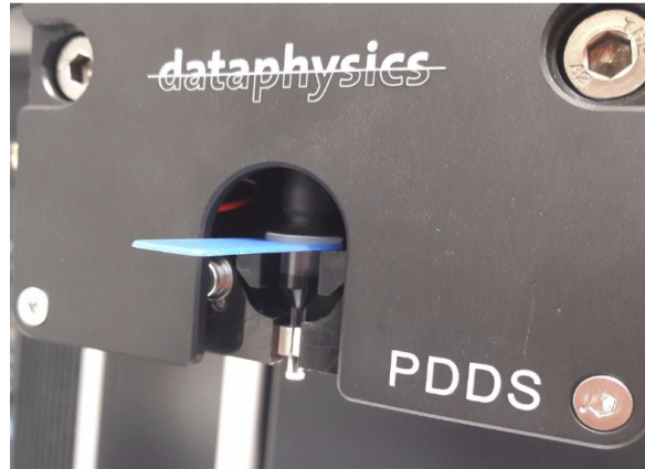
Figure 6: The cartridge is inserted into the dosing head of the picoliter head. This dosing element is positioned on the membrane cap of the cartridge, enabling to create a pulse which presses the liquid through the orifice of the cartridge.
