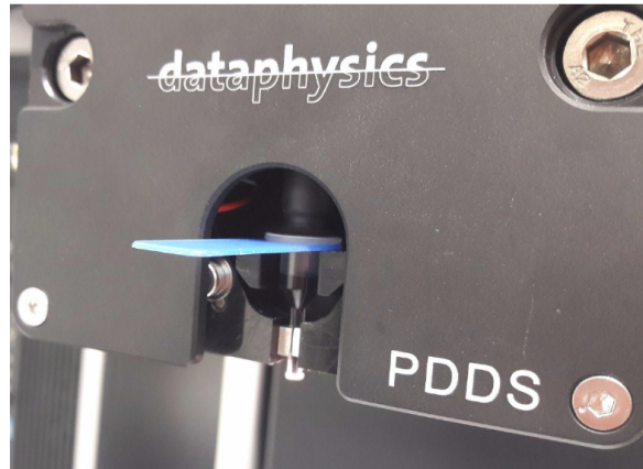
Figure 4: The cartridge is inserted into the dosing head of the picoliter head. This dosing element is positioned on the membrane cap of the cartridge, enabling to create a pulse which presses the liquid through the orifice of the cartridge.
