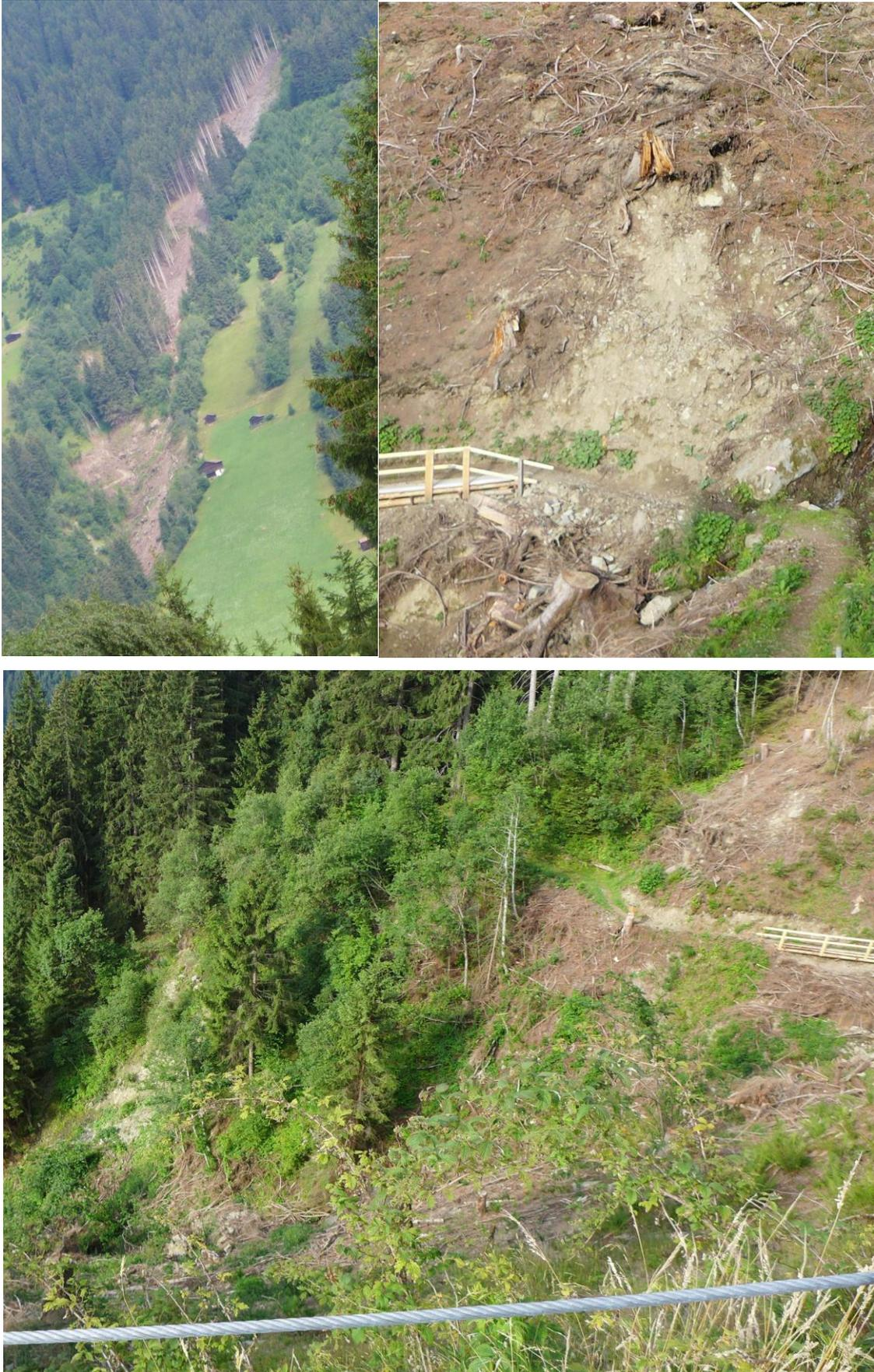
Figure 25: left: Landslide near Perfall; right: Landslide up close (Outcrop 54), with a new wooden bridge; picture below: Possible landslide continues beneath the trail; fine grained soil with blocks up to a 0.5 m. ; Outcrop 149 (referenced in the large map at the end of the thesis)
