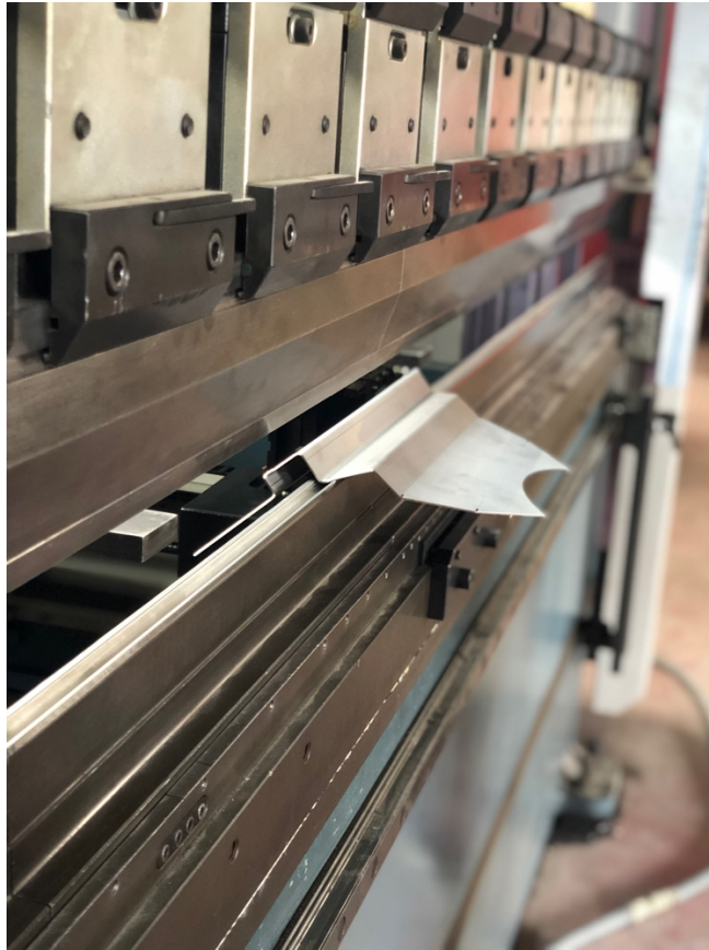
Figure 35 - Bending of the new BOWA on press (Source: Own picture)
