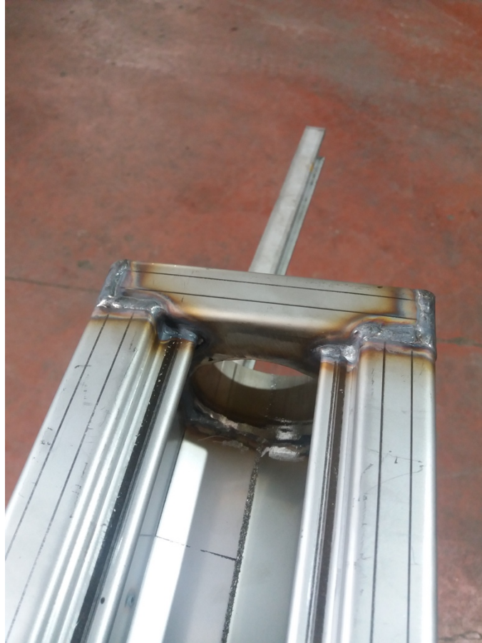
Figure 48 – Weld on both sides (Source: Own picture)
