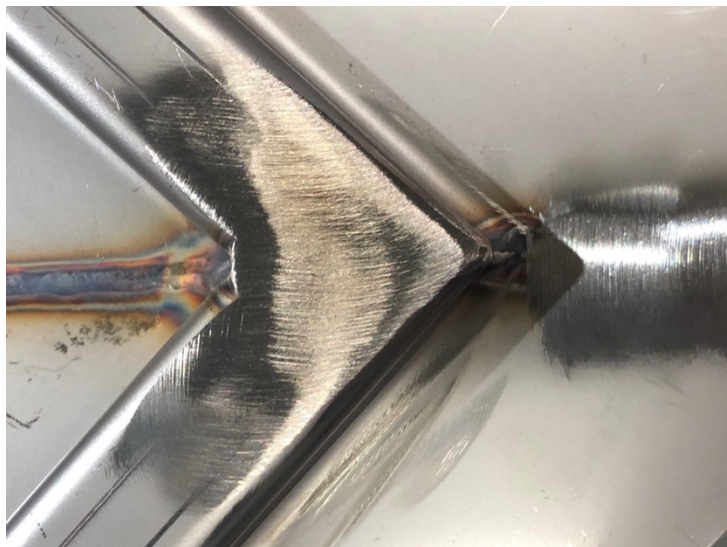
Figure 22 - Weld thickness removed (Source: Own picture)
