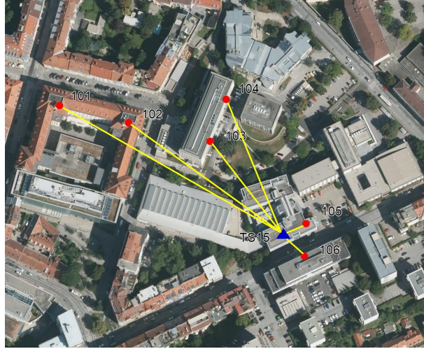
Figure 5.1: Overview of target setup, which were included during the static and dynamic ATR measurements
