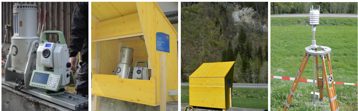
Figure 6.2: Pictures taken from the setup point and the meteo station used for the measurement campaign at Wald am Schoberpass.
