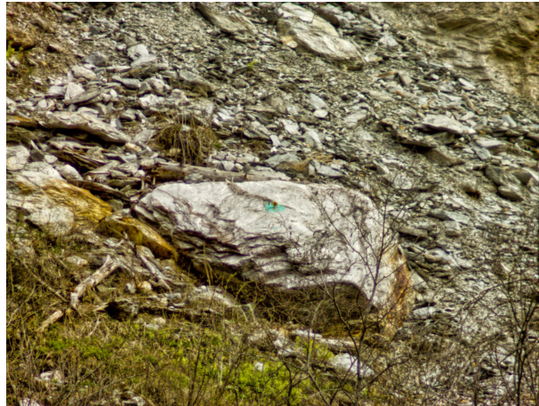
Figure 6.3: Full image of target 110, showing the mini prism installed on a single rock
