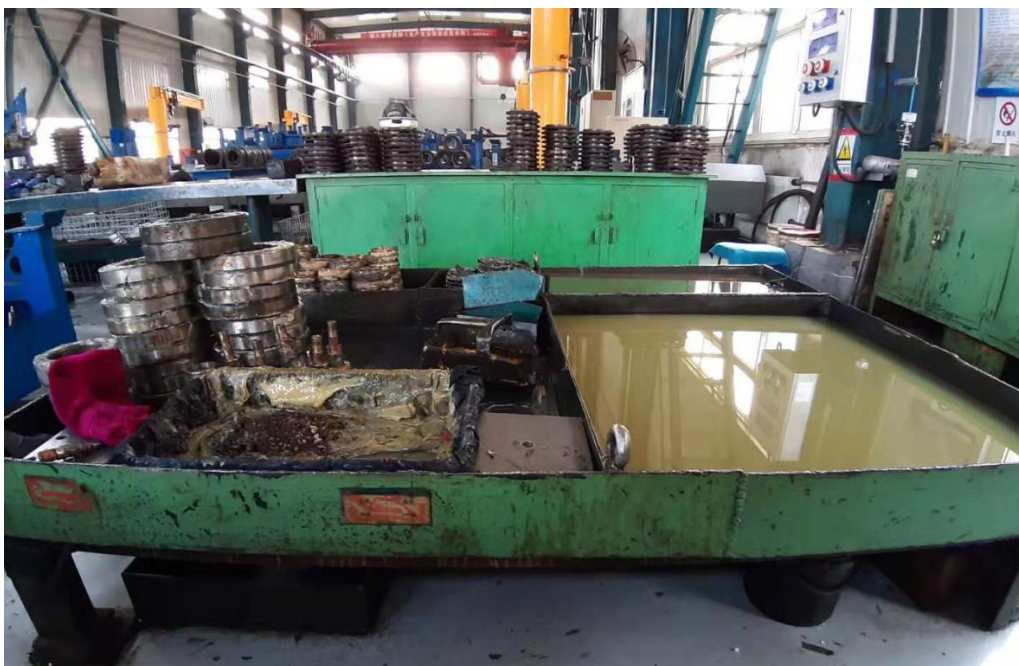
Figure 4-11: Manual cleaning station
