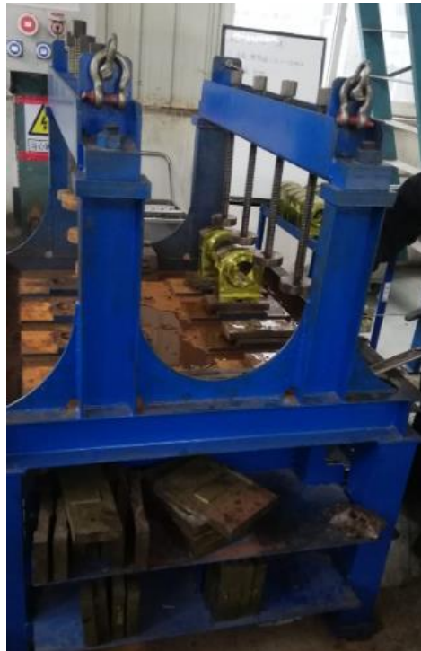
Figure 3-4: Water test table for the bearing blocks
