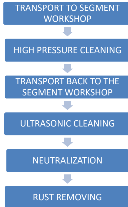
Figure 4-12: Cleaning process from January
