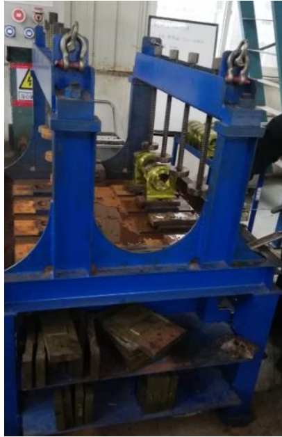
Figure 4-13: Water test table for the bearing blocks
