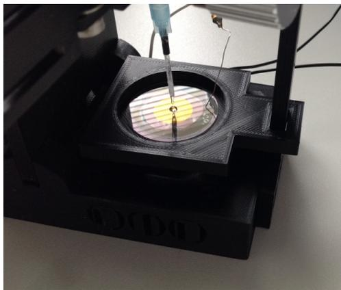
Figure 4.1.: 3D printed measurement assembly
