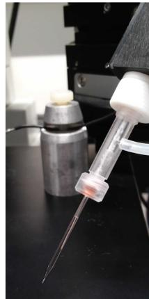
Figure 4.3.: Fully prepared measurement pipette
