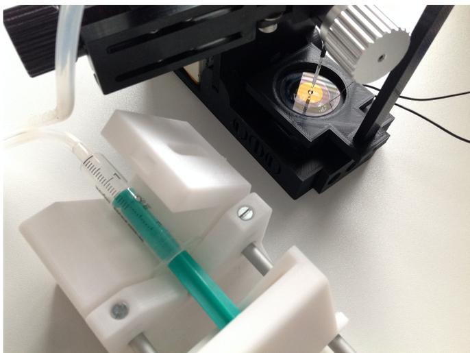
Figure 6.1.: Syringe pump for a controlled drop delivery
