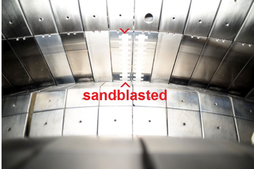
Figure 3.1.: Lower Divertor in ASDEX Upgrade, showing the higher surface roughness – therefore lower reflectivity – of the sandblasted area on the tiles [IPP18].
