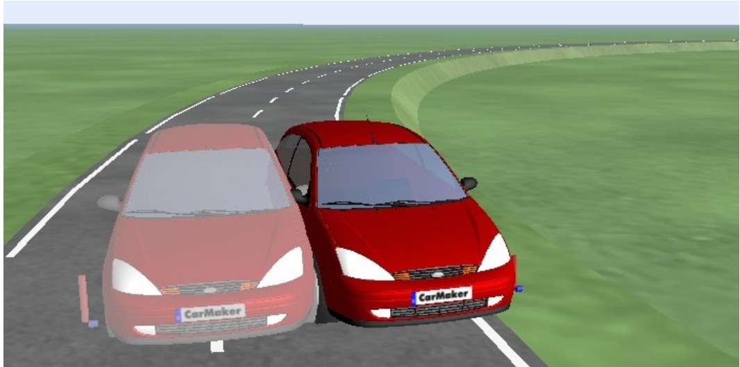
Figure 5.5: Picture of the simulation render comparing the shaded reference car and a test run car with artificial drift of 5ms.
