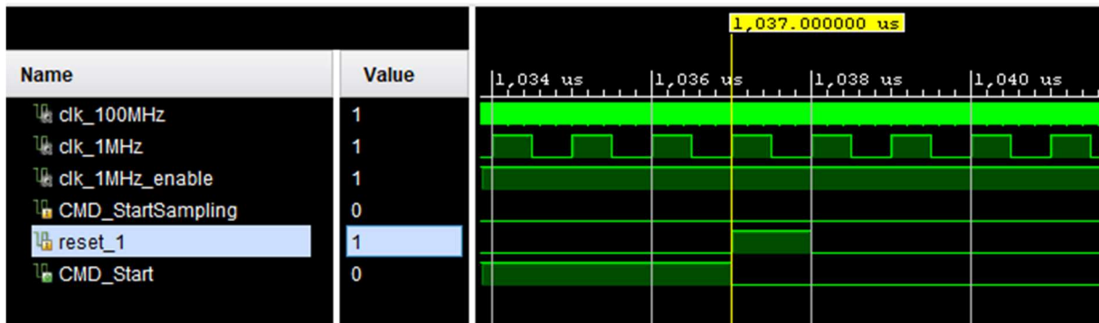
FIGURE 42: START_CONTROL SIMULATION OF THE CMD_START SIGNAL RESET
