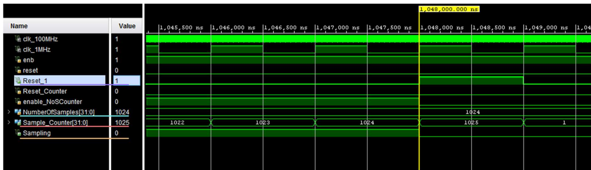
FIGURE 53: SEND_CONTROL SIMULATION WHEN THE NUMBER OF SAMPLES IS REACHED
