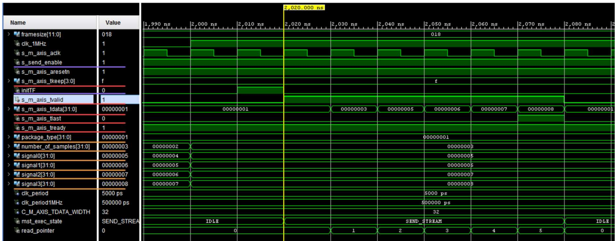
FIGURE 33: SIMULATION OF BUILDING THE AXIS DATA STREAM WITH THE PKG_SAMPLES BLOCK
