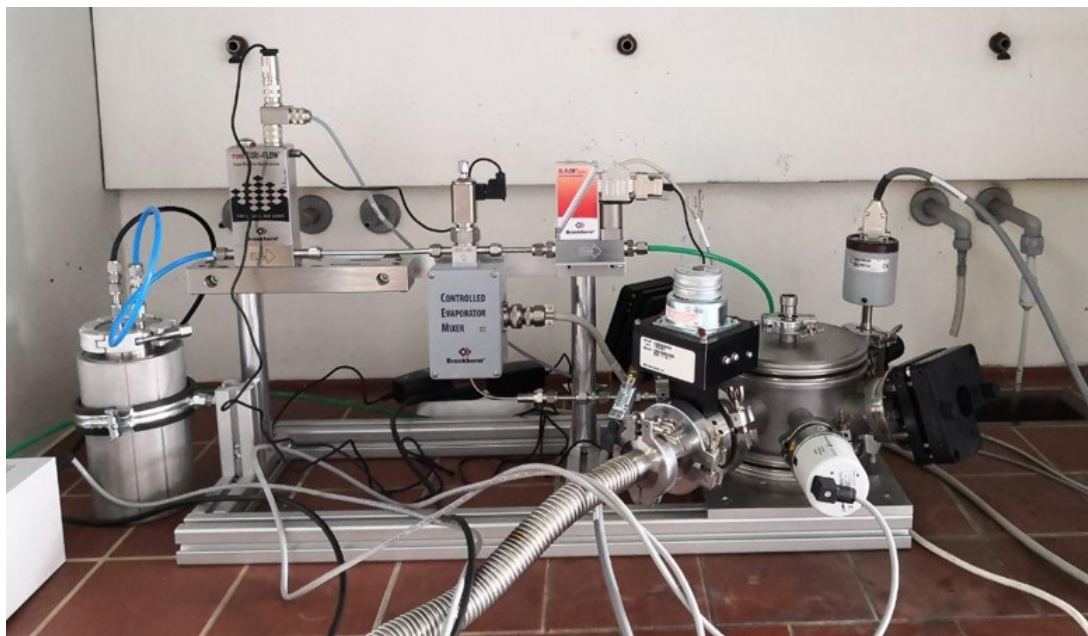
Figure 2.2: Photograph of the ellipsometric porosimeter set-up
