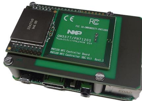
Figure 2.5: Mounted NFC shield on top of a Raspberry Pi [F3]
