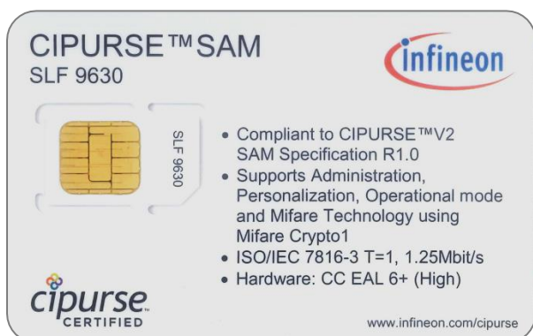
Figure 3.15: A CIPURSE™ SAM, ID-1 format on the left, ID-000 format on the right
