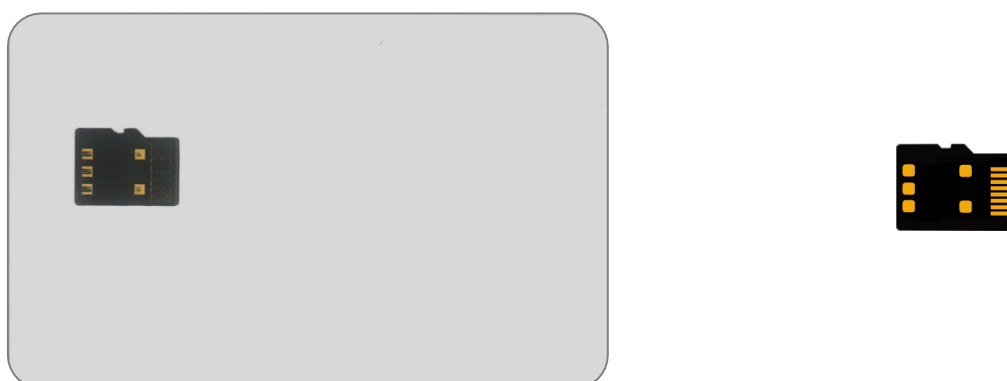
Figure 3.17: microSD card with "ISO/IEC 7816" interface (in an ID-1 form adapter on the left)
