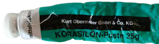
Fig. 5.4: To mount or separate both cell halves, a lubricant simplifies the process. The finally chosen lubricant is visualized.
