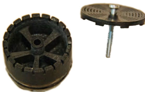
Fig. 5.1: Gravibox, a vessel for drying agent, having a removable slitted cap to provide access to humidity to pass by.
