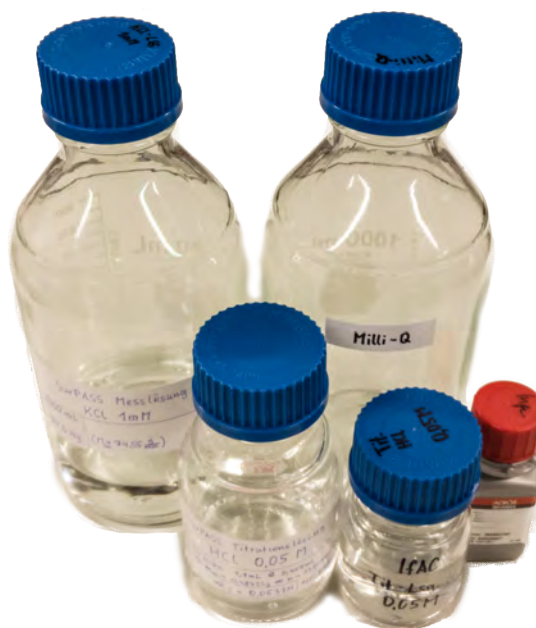
Fig. 2.11: Solutions (KCl 1 mM, HCl 50 mM, Milli-Q) to be prepared for rinsing and measuring on the SurPASS™ 3.
