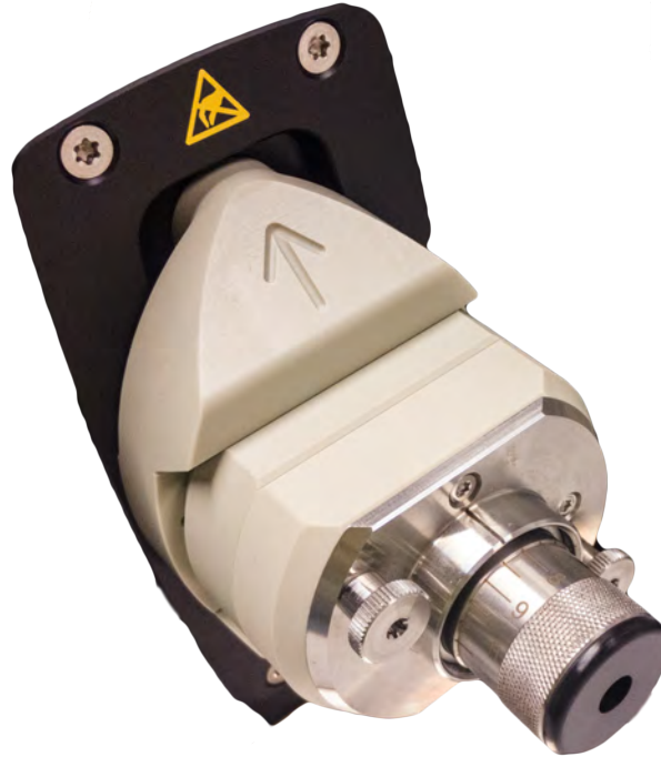
Fig. 5.12: Micrometer - 0.5 mm thread. One graduation line therefore equals 25\ \mu\text{m} .
