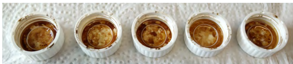
Fig. 2.6: P_4O_{10} after absorption of water shows a polyphosphorous liquid containing black residues.
