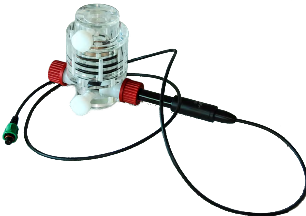
Fig. 2.8: Diffusion cell, utilized with a conductivity electrode to detect ions passed through the membrane.
