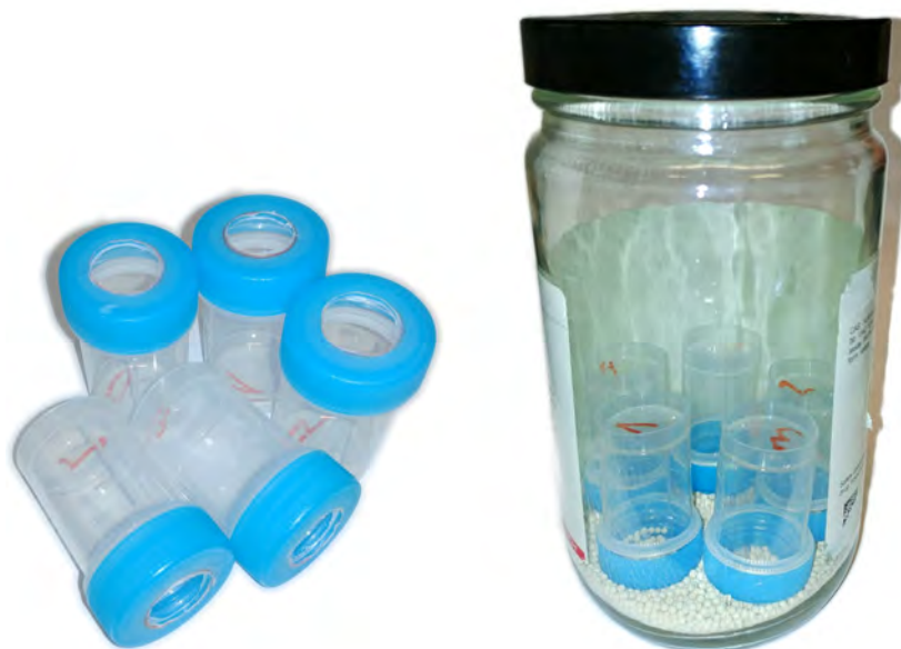
Fig. 2.5: "Rapid Analysis Cells" as predecessors for gravimetric reference analysis. Dialysis tubes are clamped in into PP vials to build a barrier for the determination of diffusion to occur. The bottle is an empty storage vessel for metallic lithium, filled with drying agent.
