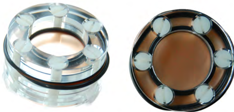
Fig. 5.3: Deformed O-rings as a result of thermal treatment in a drying cabinet.
