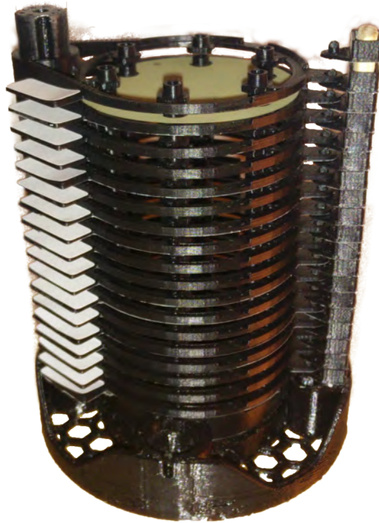
Fig. 5.2: A drying tower, providing the possibility to label and sort membranes of certain materials. In the lower part, different drying agents can be deployed. The removal of a membrane of interest is a process of ease by just unlocking and rotating the corresponding tray.
