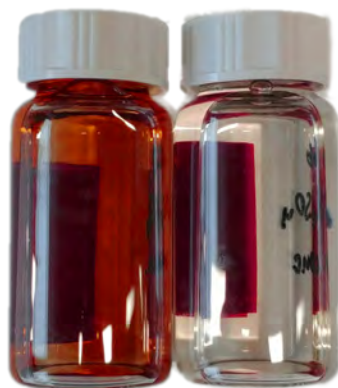
Fig. 2.10: Coloring of \text{H}_2\text{SO}_4 in presence of R1570 (dark red) and R1566 (light red). Both GREC membranes develop a reddish surface when getting immersed into concentrated sulphuric acid.
