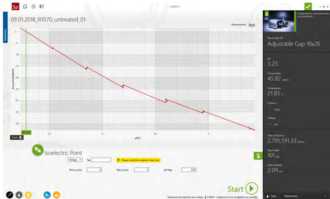
Fig. 5.14: Finished acquisition of the isoelectric point at pH 3.28.
