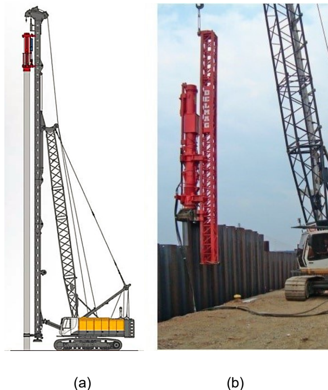
Figure 2.15 Types of crane-supported leaders for pile driving. Source: (BAUER Maschinen GmbH 2017, The Constructor 2017)
