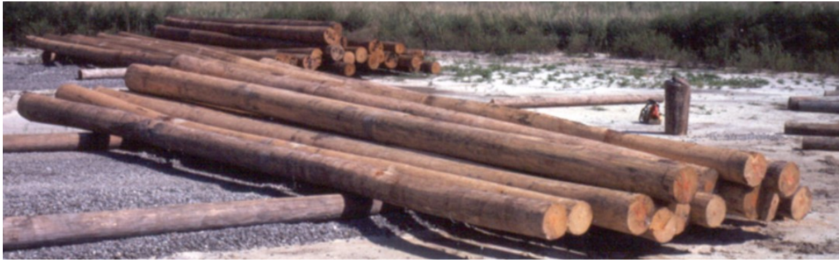
Figure 2.1 Timber piles. Source: (Hannigan et al. 2016)
