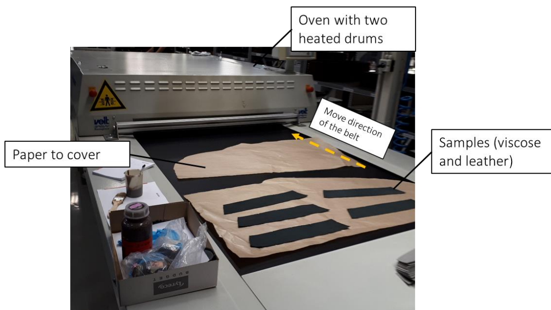
Fig. 4-35: Laminating machine with leather-viscose samples located in the seat manufacturing hall. The samples were transferred on a conveyer belt in the oven zone, where two heated drums apply a contact pressure.
