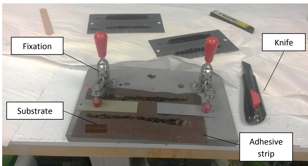
Fig. 4-4: Experimental set up for the initial adhesion test: The adhesive strip was applied onto leather and cured at 24^\circ\text{C} , 58 % r.H. for 60 min. After putting the leather sample in the fixation, the adhesive strip was removed with a knife.
