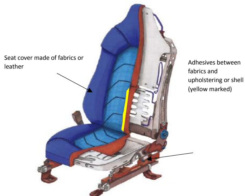
Fig. 3-5: Construction of a seat: Adhesive are applied for bonding cotton, fabric or leather to the upholstery or shell, adapted from [81].
