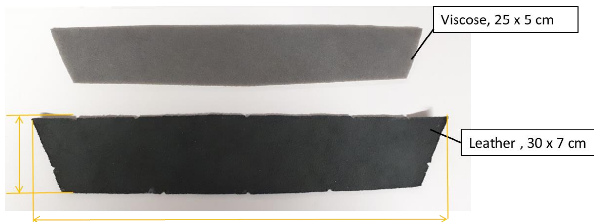
Fig. 4-34: Dimension of the leather-viscose components which used in the car seat manufacturing and were bonded on a laminating machine
