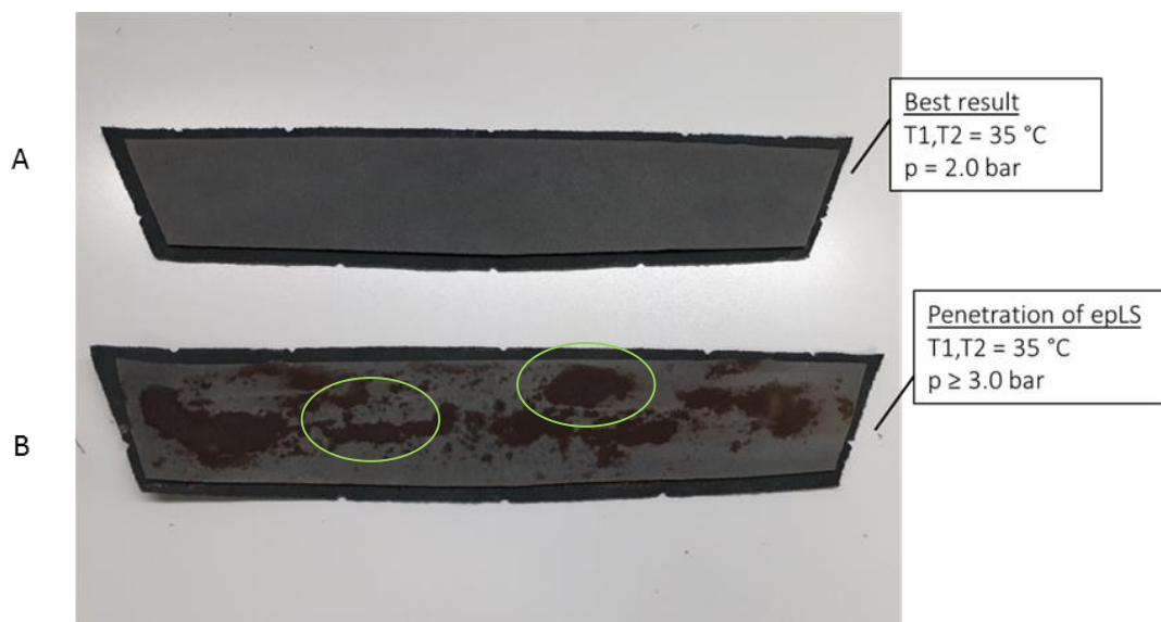
Fig. 4-37: Comparison of two leather-viscose samples, bonded with epLS-adhesive on the laminating machine: (A) showed the best result, (B) shows penetration of the epLS at p \geq 3 bar
