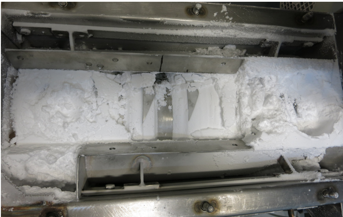
Figure 3.62.: Material at the end of test run V19 without the top half shell covers. The material deposit on the inlet was already partly removed with a vacuum cleaner.
