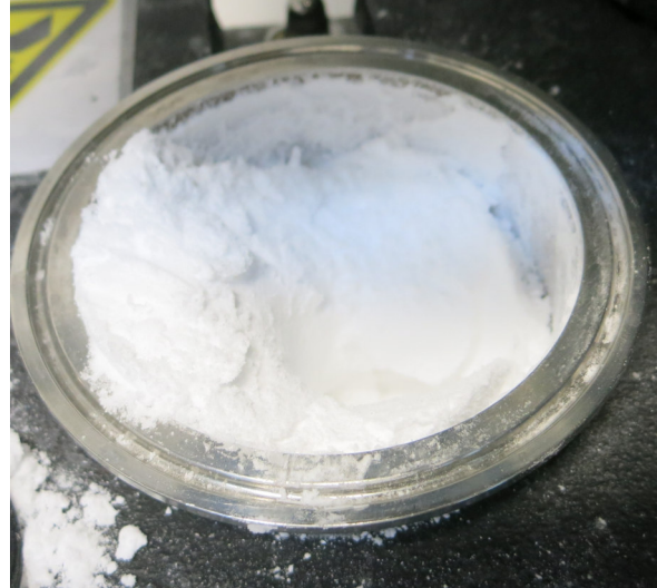
Figure 3.50.: Top view on the material deposits at the dryer inlet.
