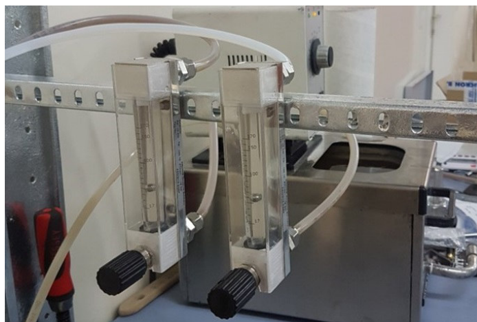
Figure 3.20.: Variable area flow meters to regulate the mass flow of hot water through the shaft and housing of the dryer.
