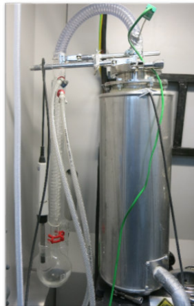
Figure 3.23.: Measurement of relative humidity and temperature of the humid exhaust air at the dryer outlet.
