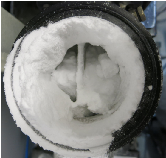
Figure 3.49.: Top view on the material deposits inside the rotary valve.
