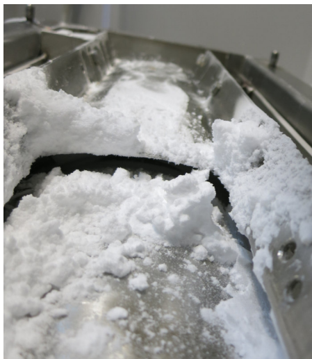
Figure 3.44.: Hollow space between half shell and shaft.
