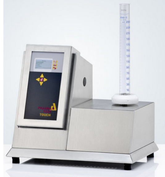
Figure 2.22.: Pharma-Test PT-TD200 tapping density and apparent volume tester. http://www.pharma-test.de/pt-td200/ (28.06.2017)
