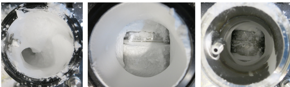
Figure 3.13.: Top view on the inlet of the dryer at the end of each test run. Left: V8 (8.4 wt.% H_2O ), mid: V7 (16.0 wt.% H_2O ), right: V9 (22.9 wt.% H_2O ).
