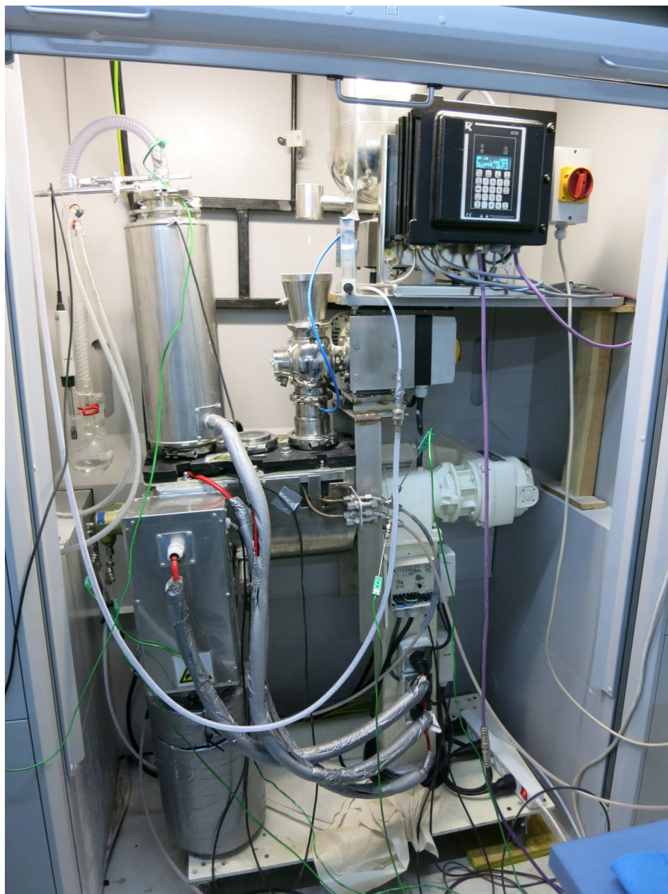
Figure 2.7.: Drying test run set up of the dryer prototype (Hosokawa)
