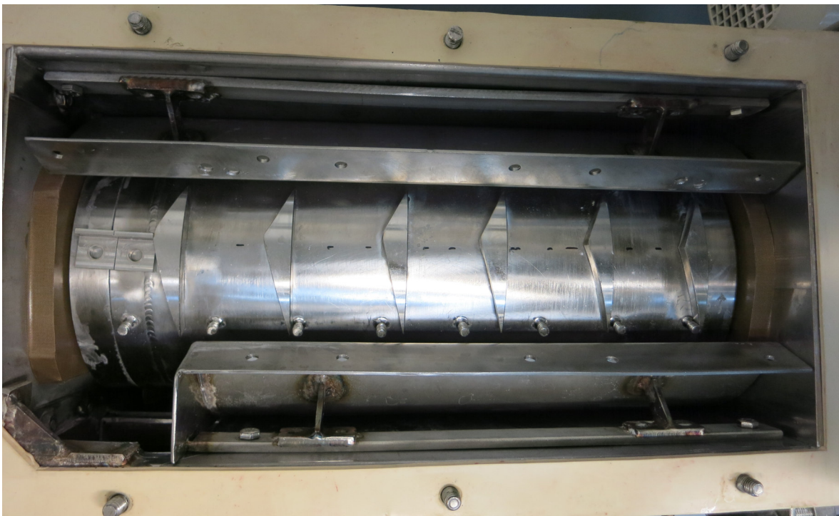
Figure 3.57.: Paddle configuration of test run V19. On the inlet and outlet side of the dryer Teflon-covered plastic plates were glued on the inner dryer wall.
