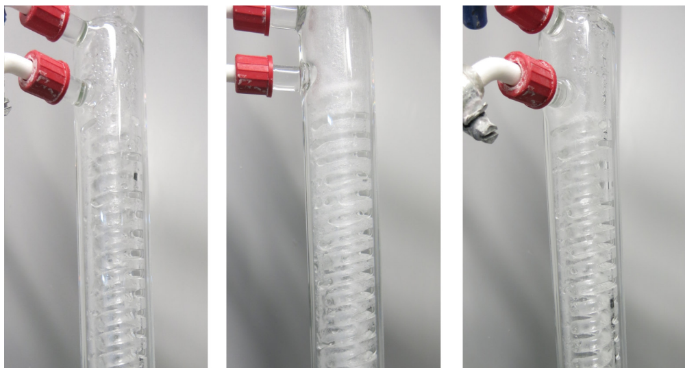
Figure 3.15.: Ibuprofen deposits in the condenser at the end of each test run. Left: V8 (8.4 wt.% H 2 O), mid: V7 (16.0 wt.% H 2 O), right: V9 (22.9 wt.% H 2 O).
