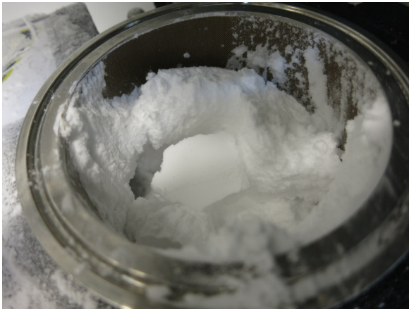
Figure 3.60.: Top view on the material deposits at the inlet of the dryer after test run V19
