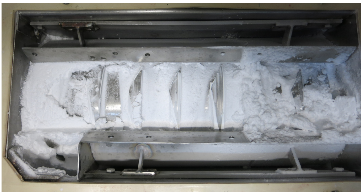
Figure 3.48.: Material inside the dryer at the end of refeed test runs V15 to V17 without top half shell covers. The material deposit on the inlet was already partly cleaned with a vacuum cleaner.
