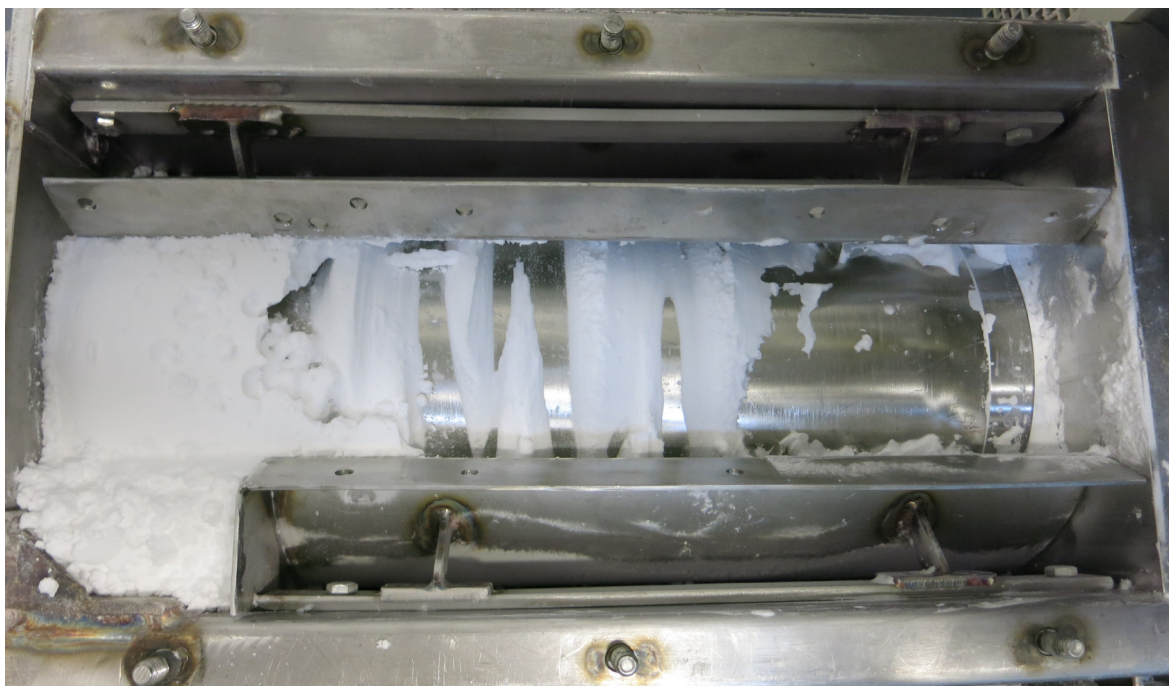
Figure 3.42.: Material inside the dryer at the end of test run V13 without top half shell covers. The material deposit on the inlet was already cleaned with a vacuum cleaner.
