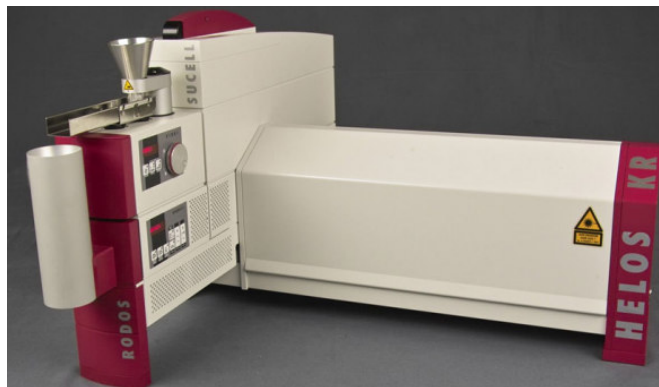
Figure 2.11.: Laser diffraction sensor HELOS/BR for dry dispersion. http://www.sympatec.com/EN/LaserDiffraction/HELOS.html (28.06.2017)
