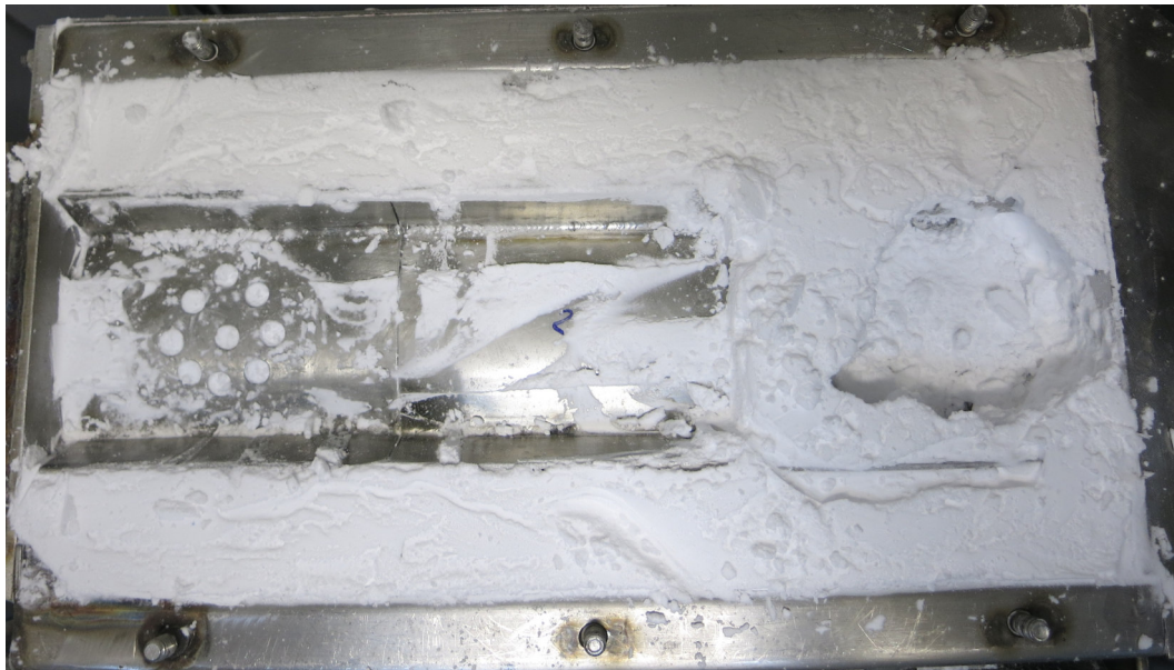
Figure 3.33.: Material inside the dryer at the end of the test run V11 with top half shell covers. Inlet and outlet part of the dryer were already cleaned with a vacuum cleaner.
