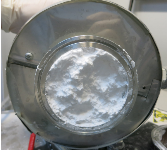
Figure 3.31.: View on the bottom side of the filter housing. The interior of the filter housing was completely filled up with Ibuprofen.
