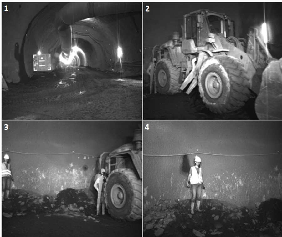
Figure 5.7: Driving into a cavern with view of a stereo camera. The person comes into camera vision at a distance of 9 metres (1-4).
