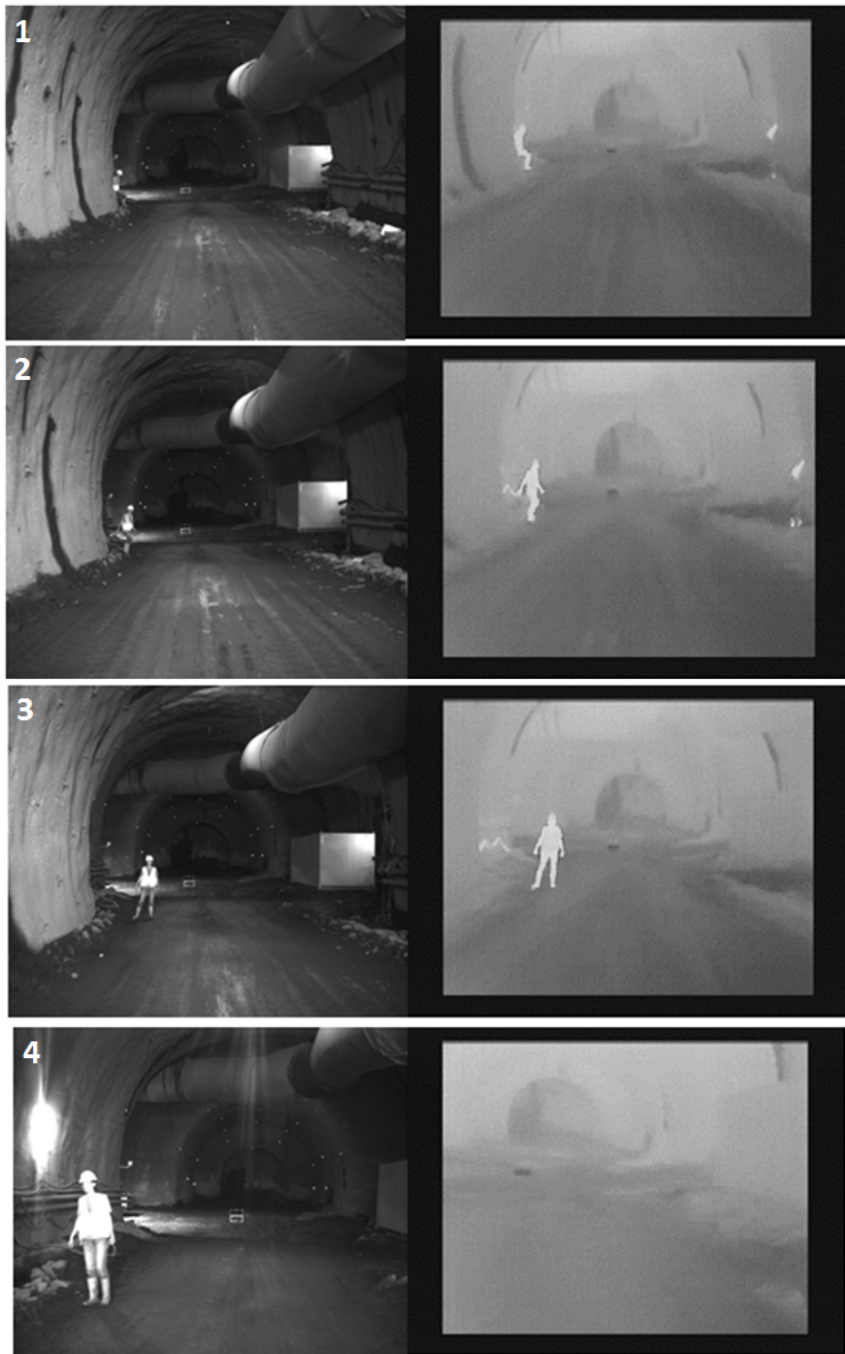
Figure 5.3: Test run process for scenario 8 (1-4). The sequence shows a person stepping out on the road, when the vehicle is 25 metres away (1) until it stops (4). The images show views from a stereo camera on the left and a thermal camera on the right side.
