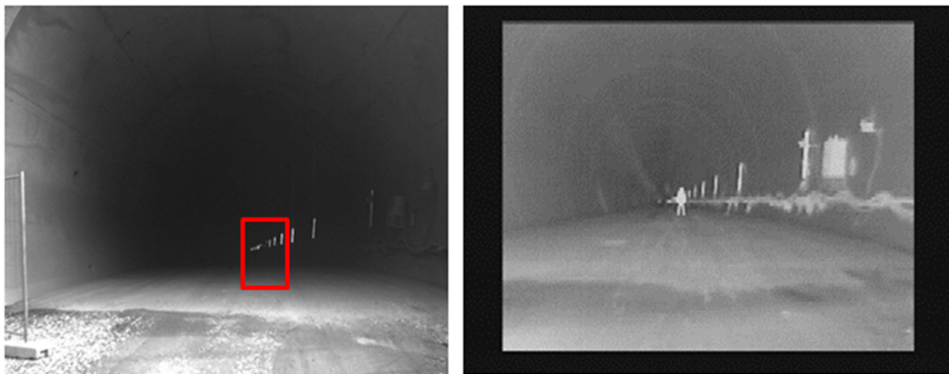
Figure 5.9: Test run for driving into a tunnel, with views from a stereo system on the left and thermal camera on the right. The person is approximately 30 metres away.
