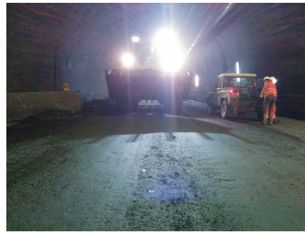
Figure 3.2: Usual front vehicle lighting for a wheel loader.
