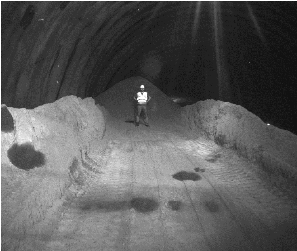
Figure 5.8: Test run for driving up a ramp, with view of a stereo camera.
