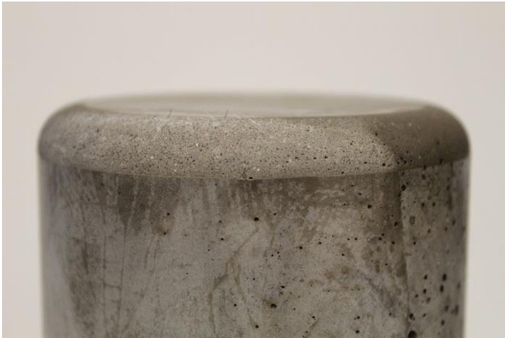
Figure 4.5: Punch 2 after the deep drawing tests
