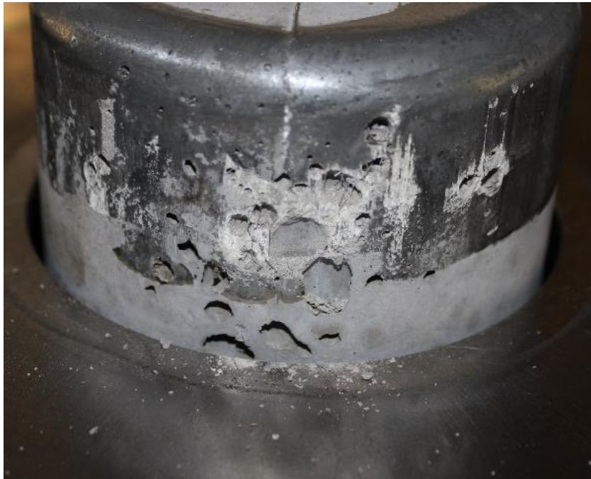
Figure 4.6: Punch 1 after the preliminary tests
