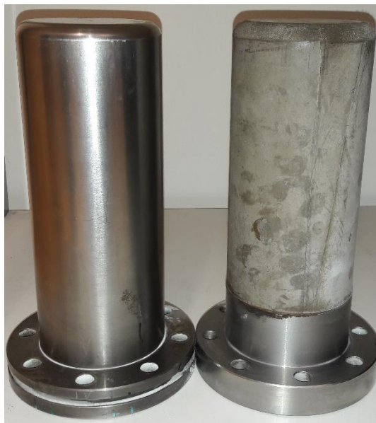
Figure 3.1: Cup geometry punch in steel and UHPC
