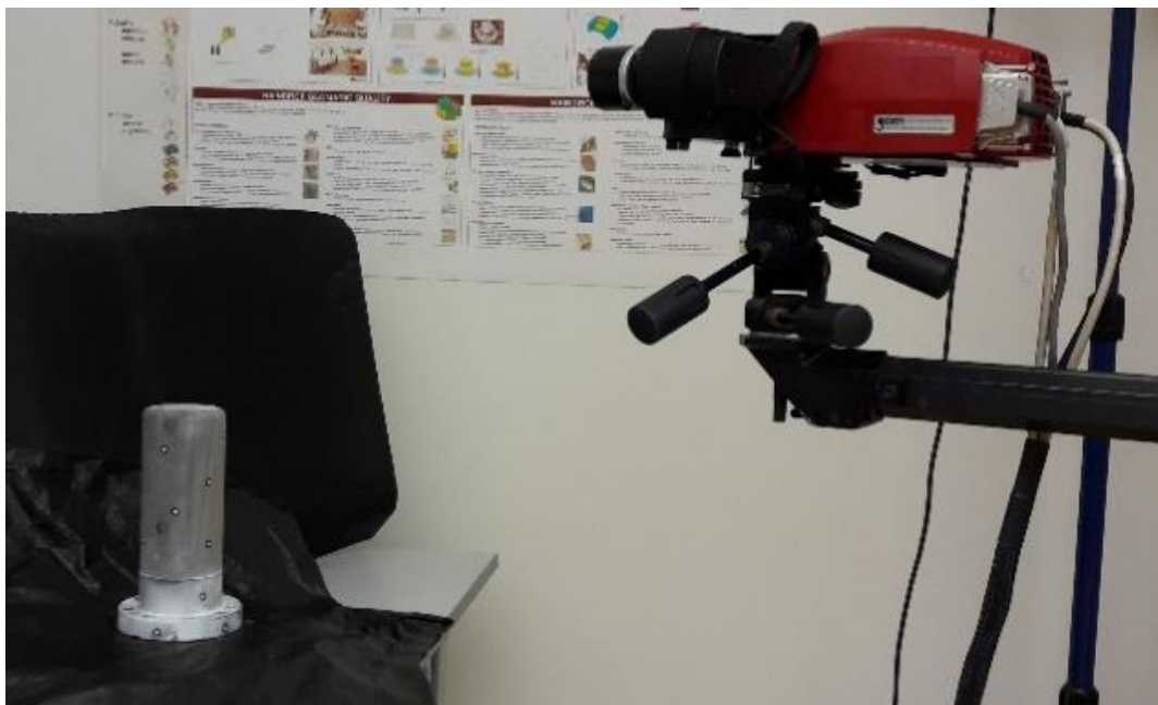
Figure 3.15: Test set up of the ATOS III 3D scanning system
