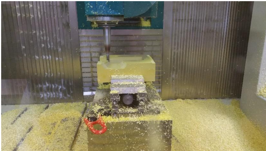
Figure 3.2: Milling of the casting mold
