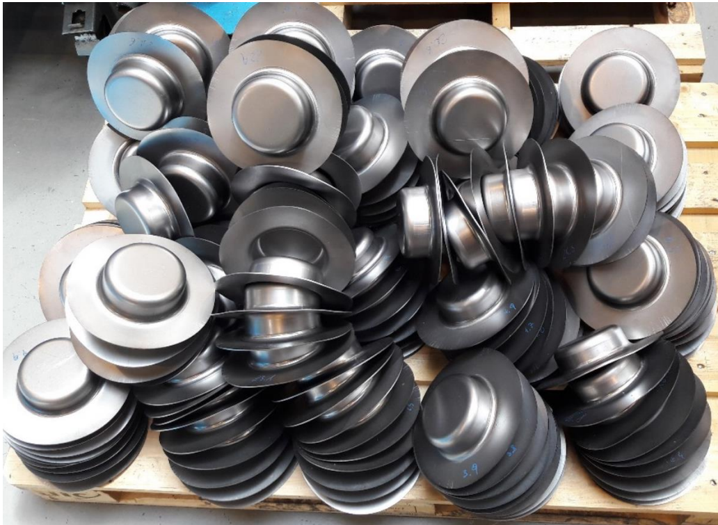
Figure 3.11: The deep drawn blanks from the main tests
