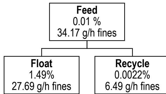
Figure 4-55 Schematic overview about the flotation process and the mass balance including consistencies at each port for bleached kraft pulp fines.
