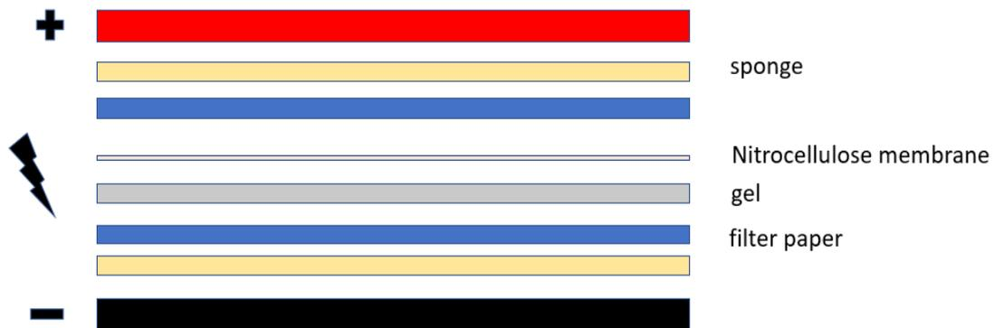
**Figure 12: Western Blot transfer cassette setup for the wet transfer.** Assembling order from top to bottom: sponge – filter paper – gel – nitrocellulose membrane – filter paper – sponge. For the wet transfer, the gel side of the sandwich is oriented toward the cathode (black), while the membrane side is positioned toward the anode (red).
