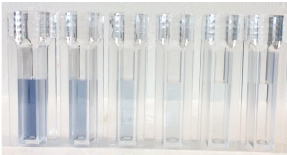
Figure 13: Calibration for the Folin & Ciocalteu assay. Gallic acid was used as standard substance.
