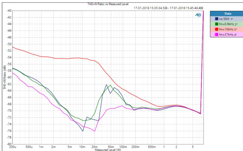
Figure 5.10.: Measured THD+N for three different SSM settings.
