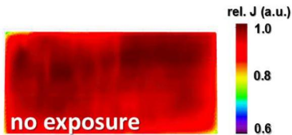
**Figure S1.** LBIC map of the area (1.5 mm x 4.0 mm) of a fresh device before any exposure (0 min).
