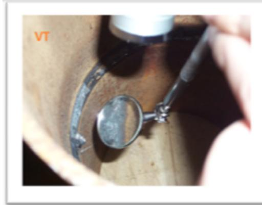
Figure 3: Example of Visual testing VT [14].
