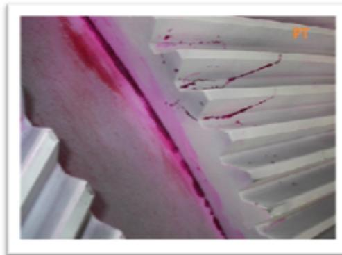
Figure 4: Example of Penetrate testing PT [8].
