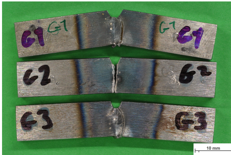
Figure A9: Butt weld Gleeble-PWHT Charpy V-notch samples after applying impact test at -20^{\circ}\text{C} .
