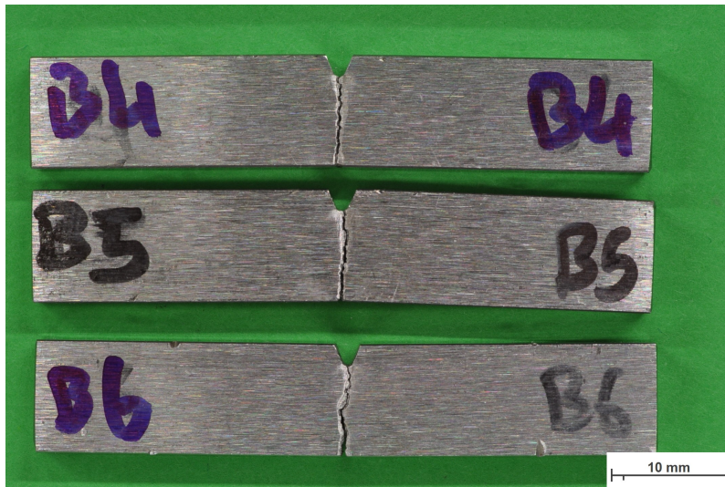
Figure A6: Butt weld EBLPWHT (B) Charpy V-notch samples after applying impact test at -40^{\circ}\text{C} .
