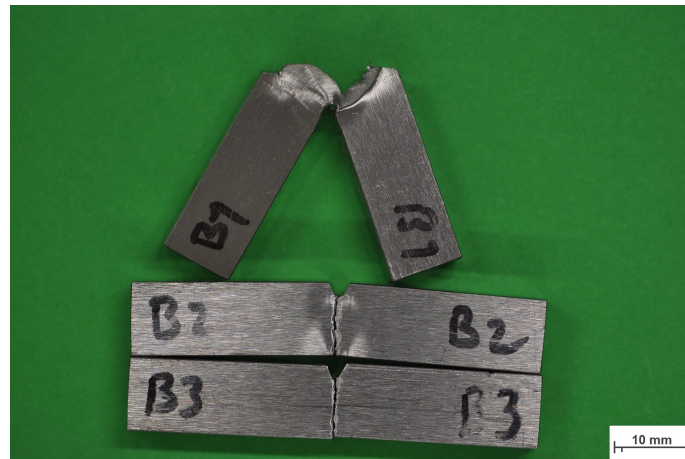
Figure 38: 3 Charpy V-notch samples after applying impact test, the first sample B1 shows fracture path deviation.
