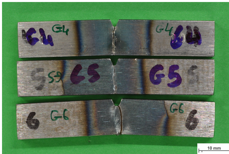
Figure A10: Butt weld Gleeble-PWHT Charpy V-notch samples after applying impact test at -40^{\circ}\text{C} .
