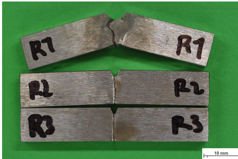
Figure A1: Butt weld as welded Charpy V-notch samples after applying impact test at -20^{\circ}\text{C} .
