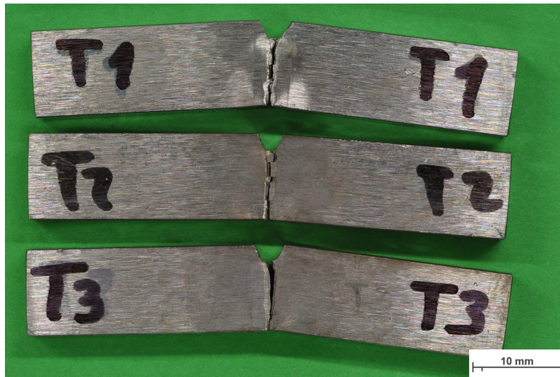
Figure A3: Butt weld EBLPWHT (T) Charpy V-notch samples after applying impact test at -20^{\circ}\text{C} .
