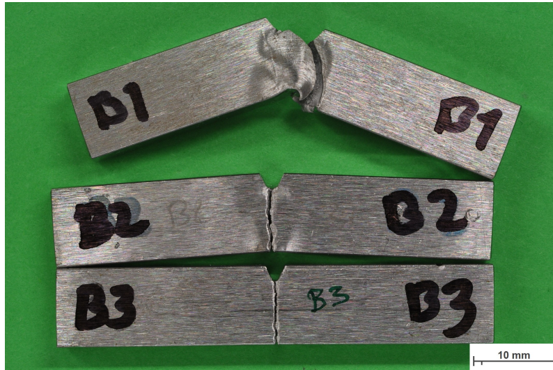
Figure A5: Butt weld EBLPWHT (B) Charpy V-notch samples after applying impact test at -20^{\circ}\text{C} .
