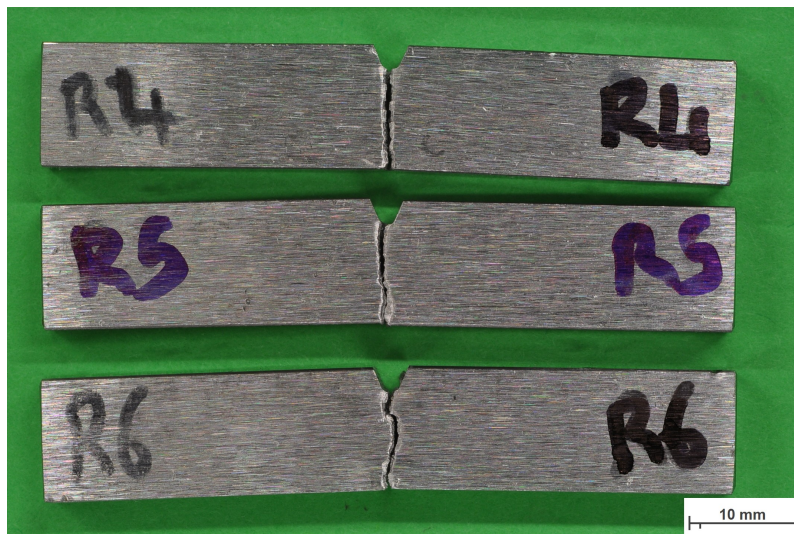
Figure A2: Butt weld as welded Charpy V-notch samples after applying impact test at -40^{\circ}\text{C} .
