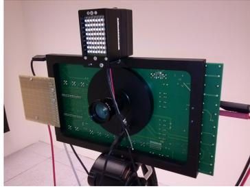
Figure 6.1: Imager setup. Sensor is central on the board with optics. The LED illumination is positioned above the sensor.
