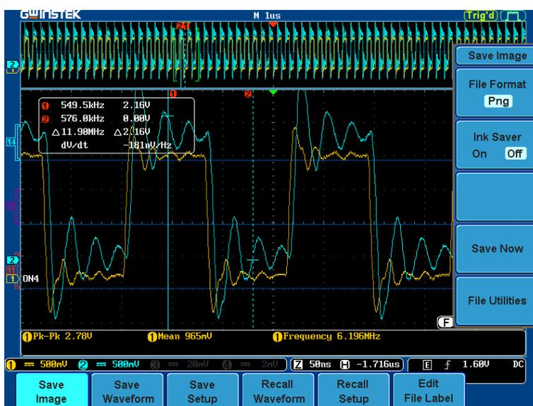
Figure 4.6: Ringing on SoundWire connection
