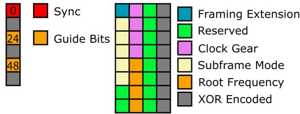
Figure 2.7: SLIMBus Control Structure
