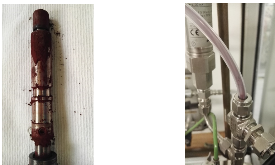
Figure 43: Catalyst coated magnetic axel after the reaction. The visible part is installed in the bearing room section where theoretically no catalyst should be present. The second picture shows the exhaust PTFE-hose. The slight red color is an indicator for the presence of finest catalyst particles in the exhaust gas stream.
