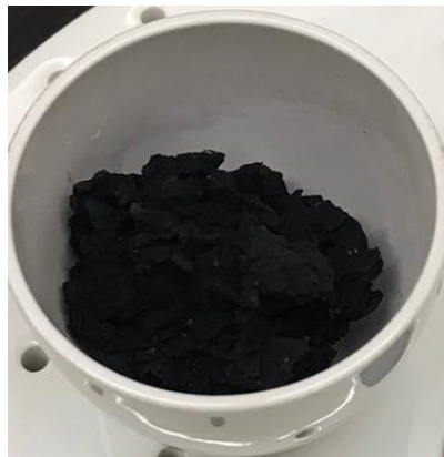
Figure 15: The figure shows the catalyst after the calcination step. The previously turquoise particles have become black.
