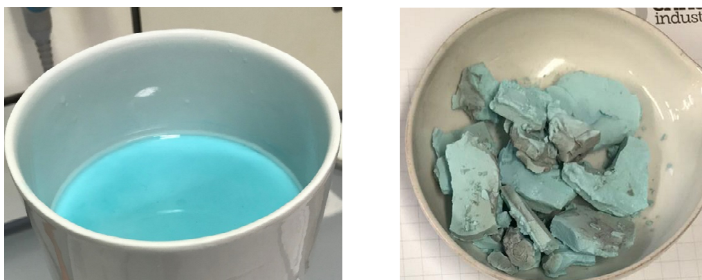
Figure 13: The picture on the left shows the turquoise catalyst precursor filter cake, while the right picture shows it after the drying process.
