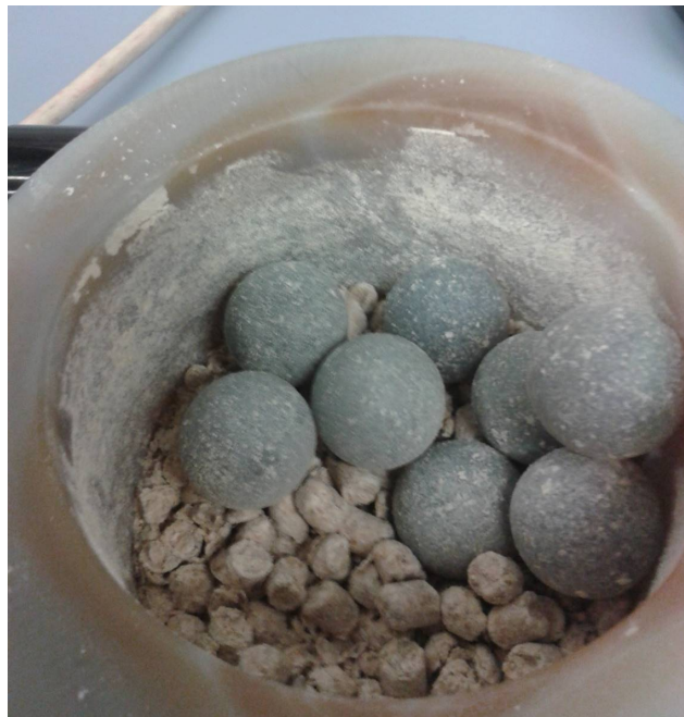
Figure 4.4: 57.8 g of 7 wt% xanthan gum cat litter after milling for 1 min in a 200 mL milling cup with milling balls (both made from agate stone).
