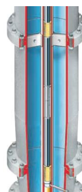
Figure 61: Enclosed line-shaft (Flowsolve corporation – VTP, 2014)
