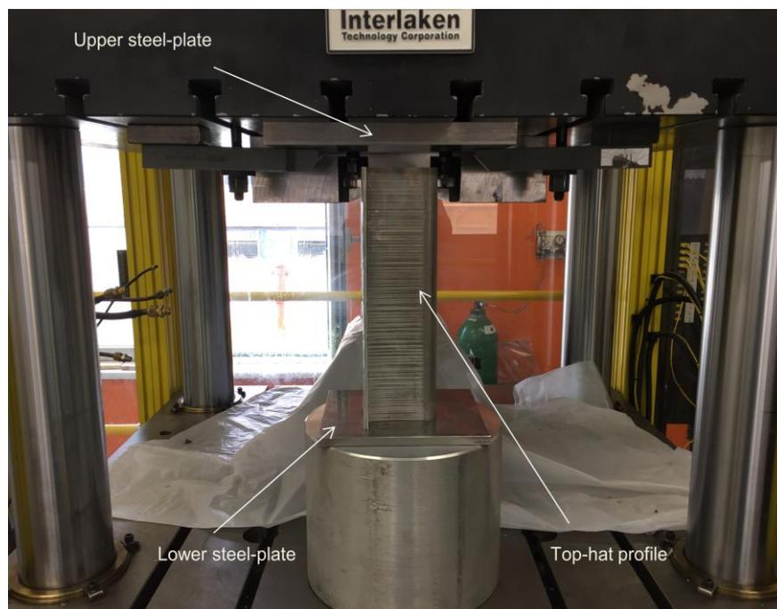
**Figure 4-13:** Test setup used for quasi-static crush testing
