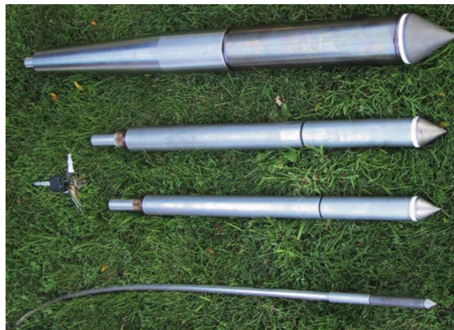
FIGURE 3.3: CPT probes with different projected area of the cone A_c . From bottom: 2 cm 2 , 10 cm 2 , 15 cm 2 and 40 cm 2 [11]
