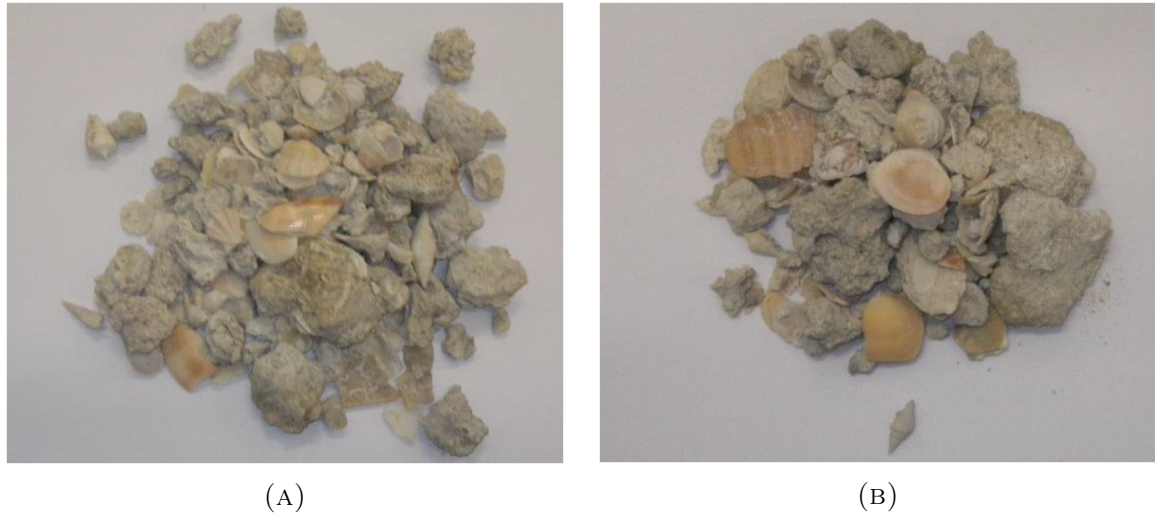
FIGURE 6.6: Sand grains larger than d > 8 mm removed from the AZ28 (A) and BC36 (B) sample [34]
