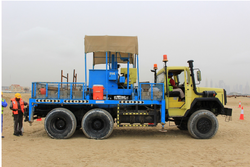
FIGURE 3.4: CPT rig as it was used on the PLM site in Dubai, UAE
