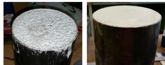
Figure 21: Add the compensation layer (gypsum) [6]
