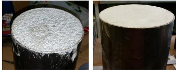
Figure 13: Filling material shrinkage (left) [6], Compensation layer (right) [6]
