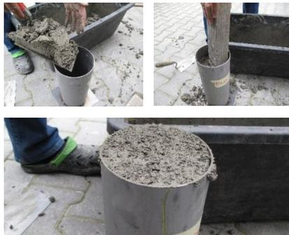
Figure 20: Fill the inner pipe with the porous filling material and compact it in layers
