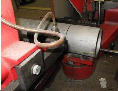
Figure 16: Cut inner and outer pipe to length
