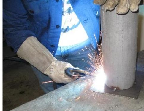
Figure 17: Weld pipe with end plate
