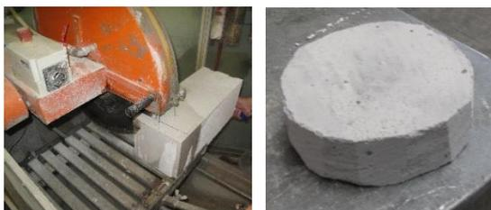
Figure 22: Shape the porous inlay
