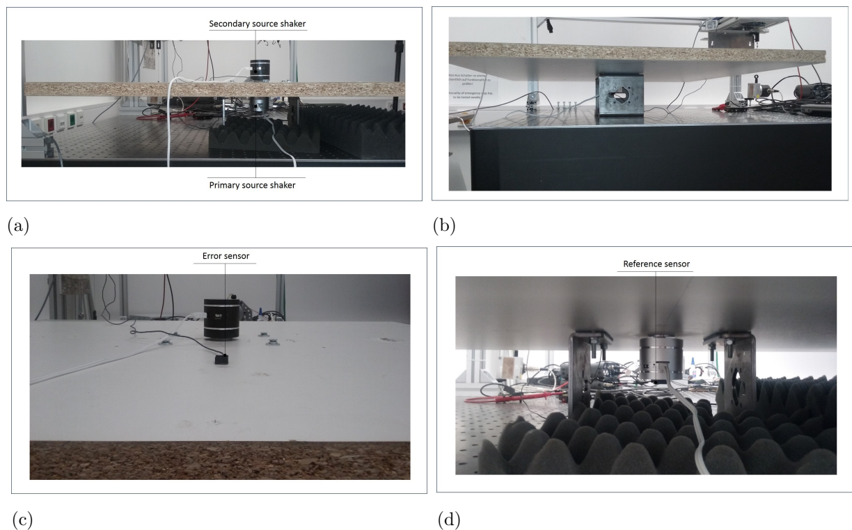
Figure 4.13: Second experimental set-up. (a) Front side. (b) Right side. (c) Top. (d) Bottom.
