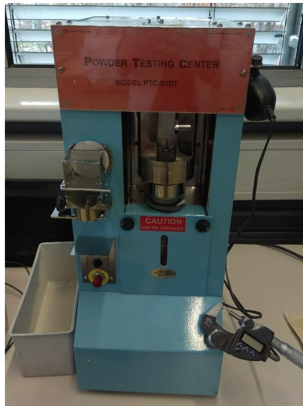
Figure 21: The PTC-03DT universal powder tester by KZK Powder Tech Corp.
