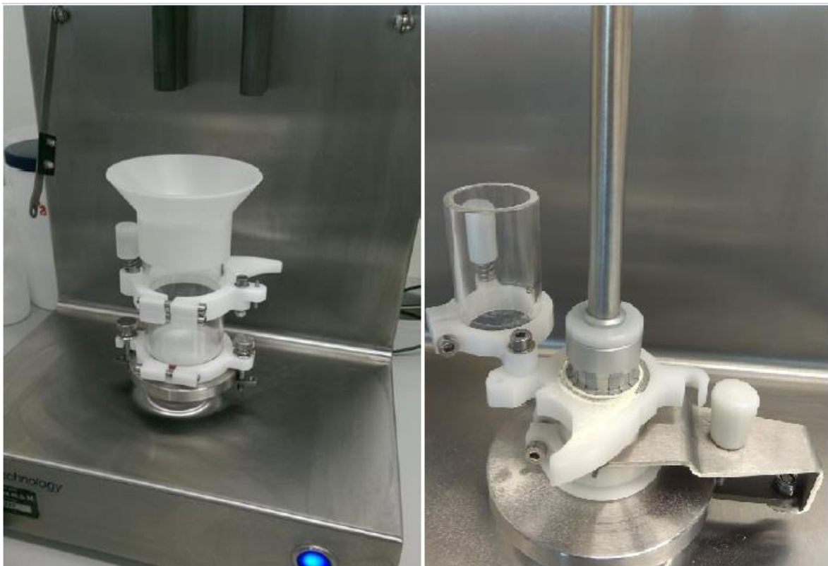
Figure 17: Shear cell preparation setup on the left; shear test in progress on the right
