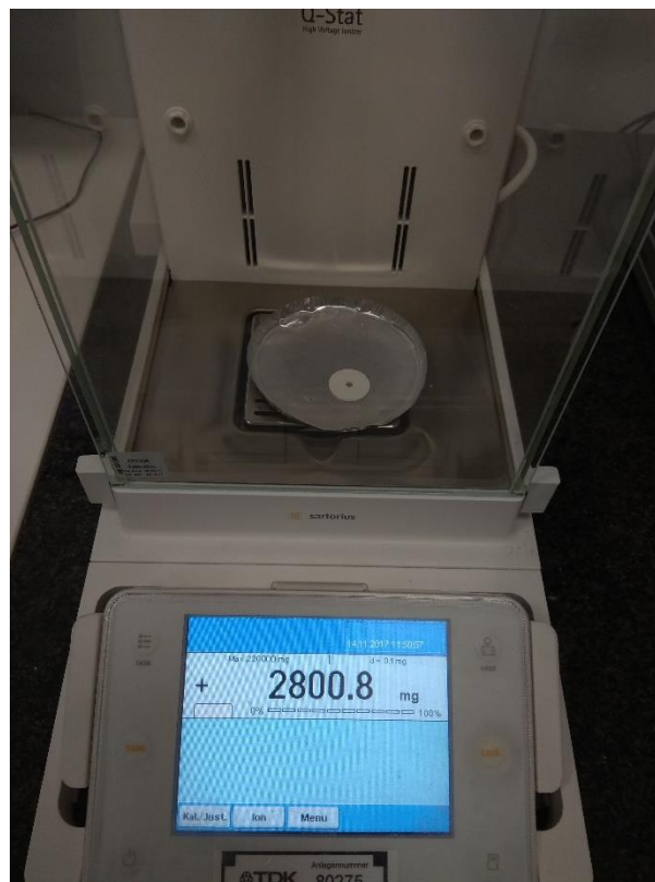
Figure 30: Green part weight measurement setup
