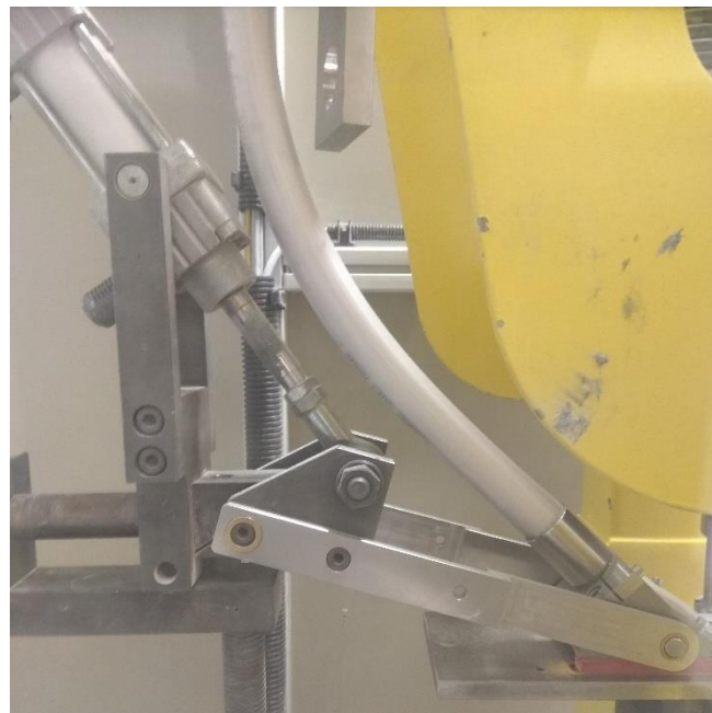
Figure 35: Filling shoe mount and actuation setup
