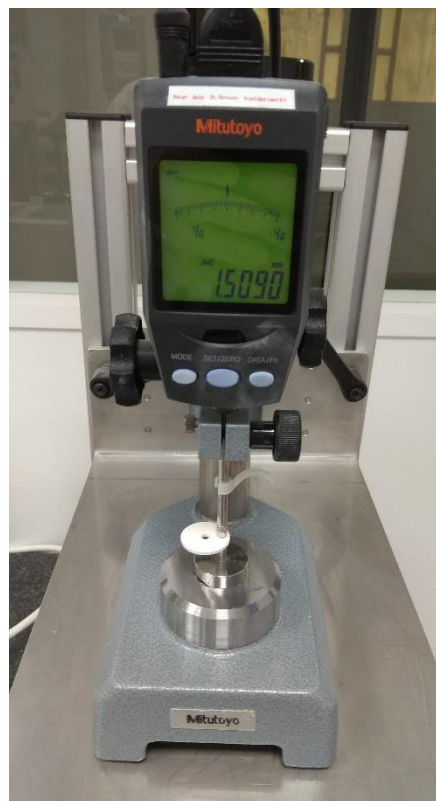
Figure 25: Height measurement setup using a dial gauge and comparator stand with a clamped green part
