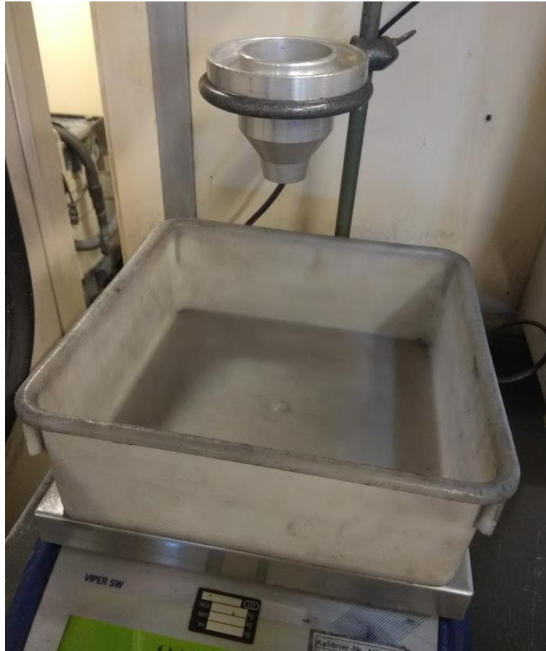
Figure 20: Flow cup viscometer measurement setup
