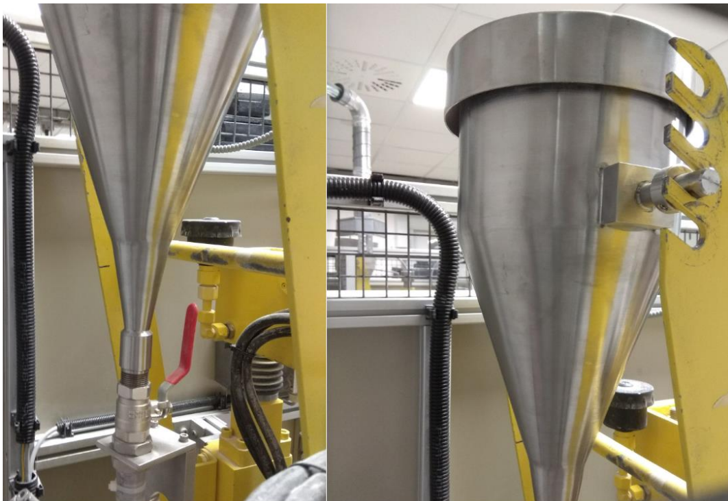
Figure 33: Funnel valve connection on the left, funnel bearing setup on the right
