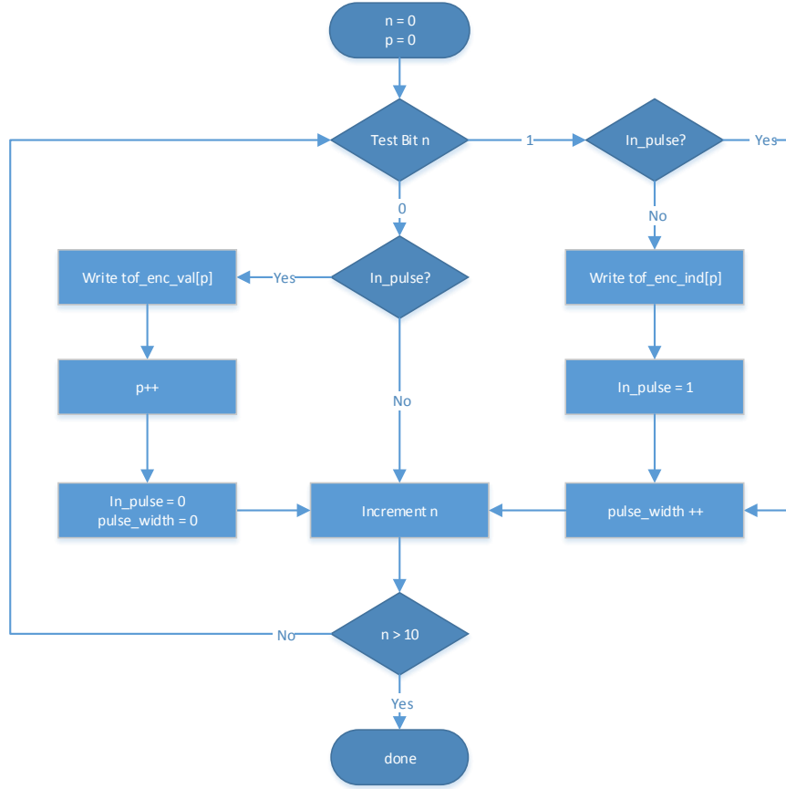
Figure 4.3: Flowchart of the transition encoder algorithm. It analyzes a 10bit input stream and detects pulse start indexes and their width in it.
