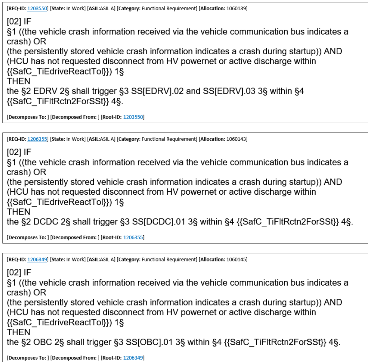
Figure 4.3: Exemplary similarities of functional safety requirement on element level based on a template [4]
