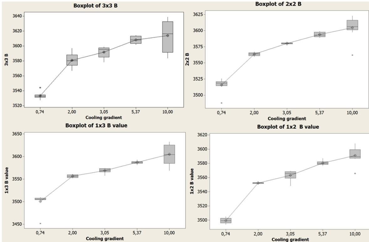
Figure 70: Influence of cooling rate on different non-standard chips: 1x2, 1x3, 2x2 and 3x3 mm<sup>2</sup>
