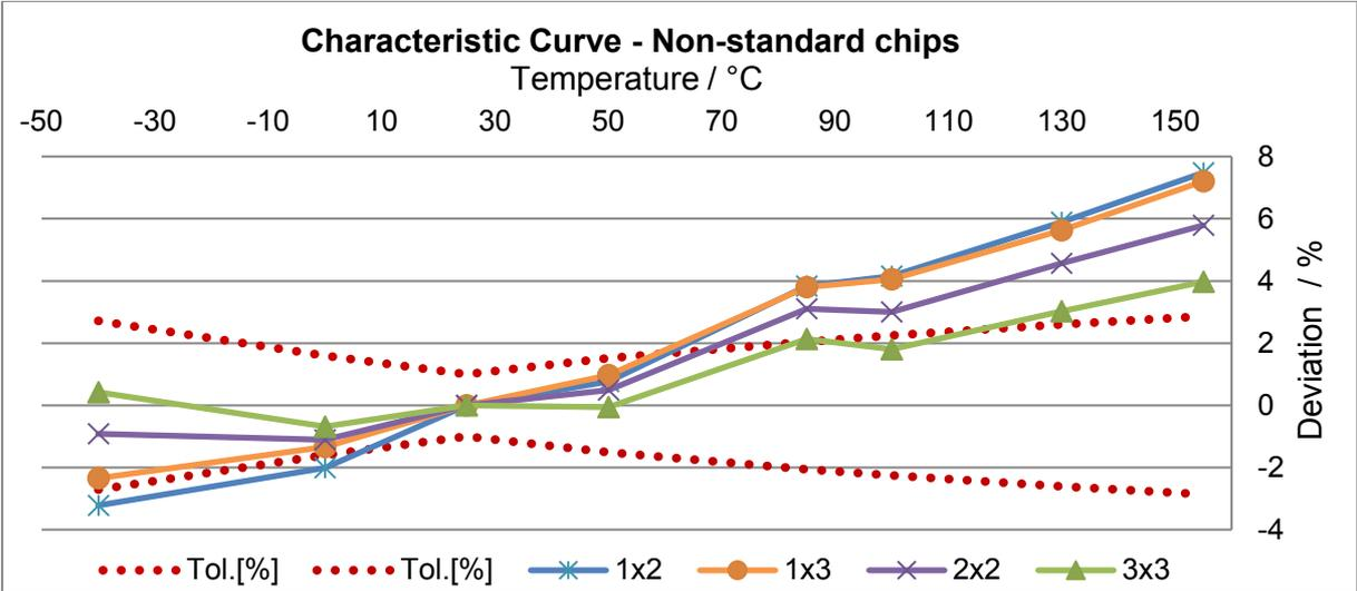
Figure 50: Characteristic curve of non-standard chips: 1x2, 1x3, 2x2, 3x3 mm<sup>2</sup>
