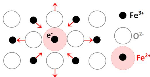
Figure 10: An electron surrounded by a deformed area of the lattice (phonon cloud). e.g. distortion created by the reduction of  $Fe^{3+}$  to  $Fe^{2+}$  (the same metal ion in two different valence states)
