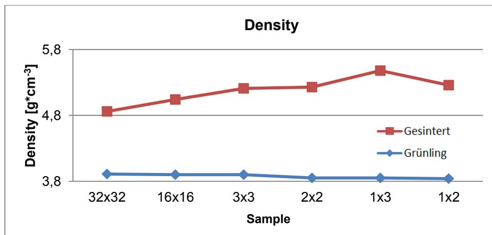
Figure 46: Calculated geometric density of green and sintered bodies
