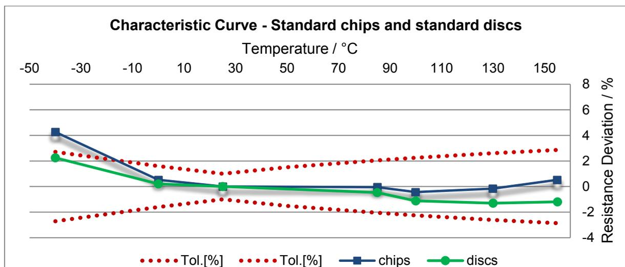
Figure 1: Resistance deviation of chips and disc made of the same material composition
