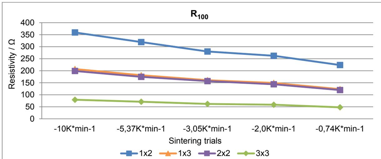
Figure 69: Evaluation of  $R_{100}$  with different cooling rates
