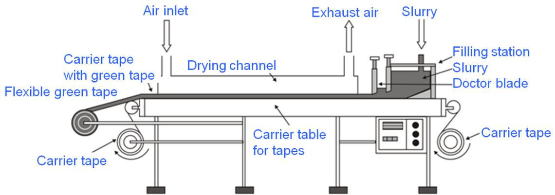
Figure 16: Layout of a continuous tape casting process (training material which has been kindly provided by TDK)
