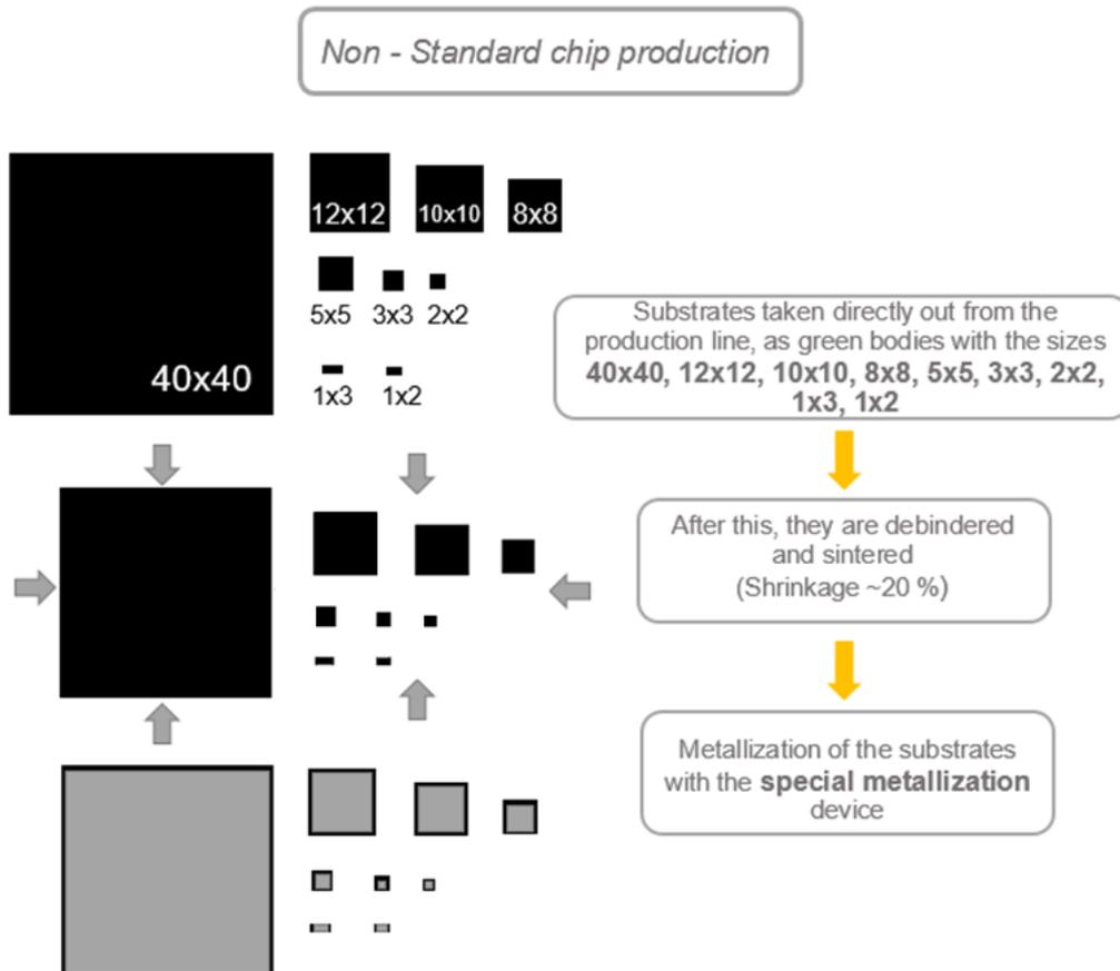
Figure 24: Non-standard chip production
