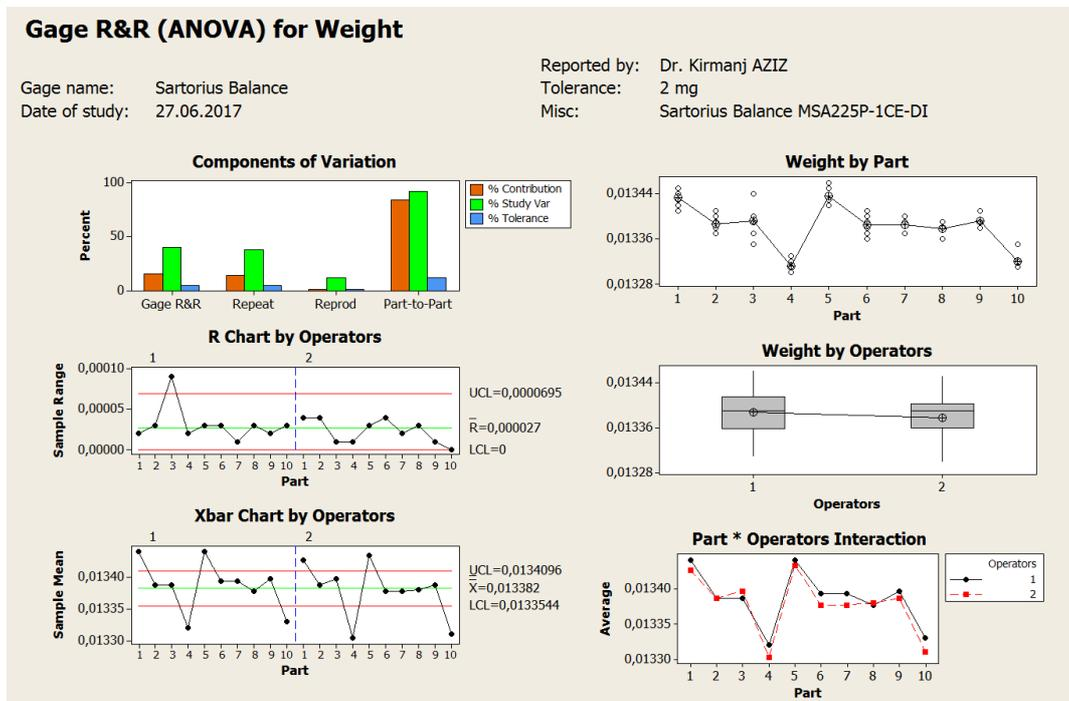
Figure 41: Graphical summary of the *Gage R&R* for the laboratory balance
