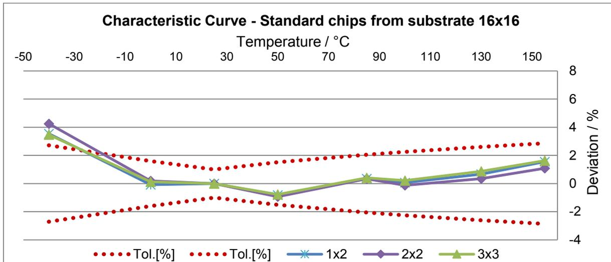
Figure 48: Characteristic curves of standard chips: 1x2, 2x2, 3x3 mm<sup>2</sup> cut from standard substrate 16x16 mm<sup>2</sup>
