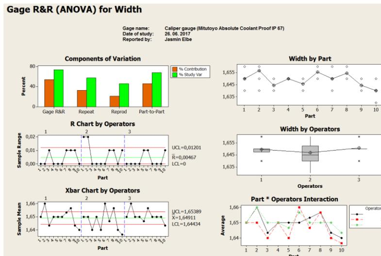
Figure 35: Graphical summary of the Gage R&R for the caliper gauge for the width
