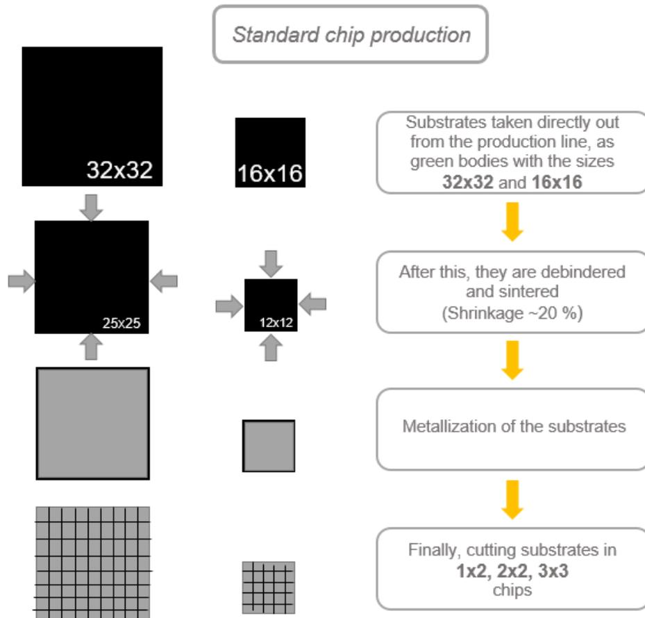
Figure 23: Standard chip production
