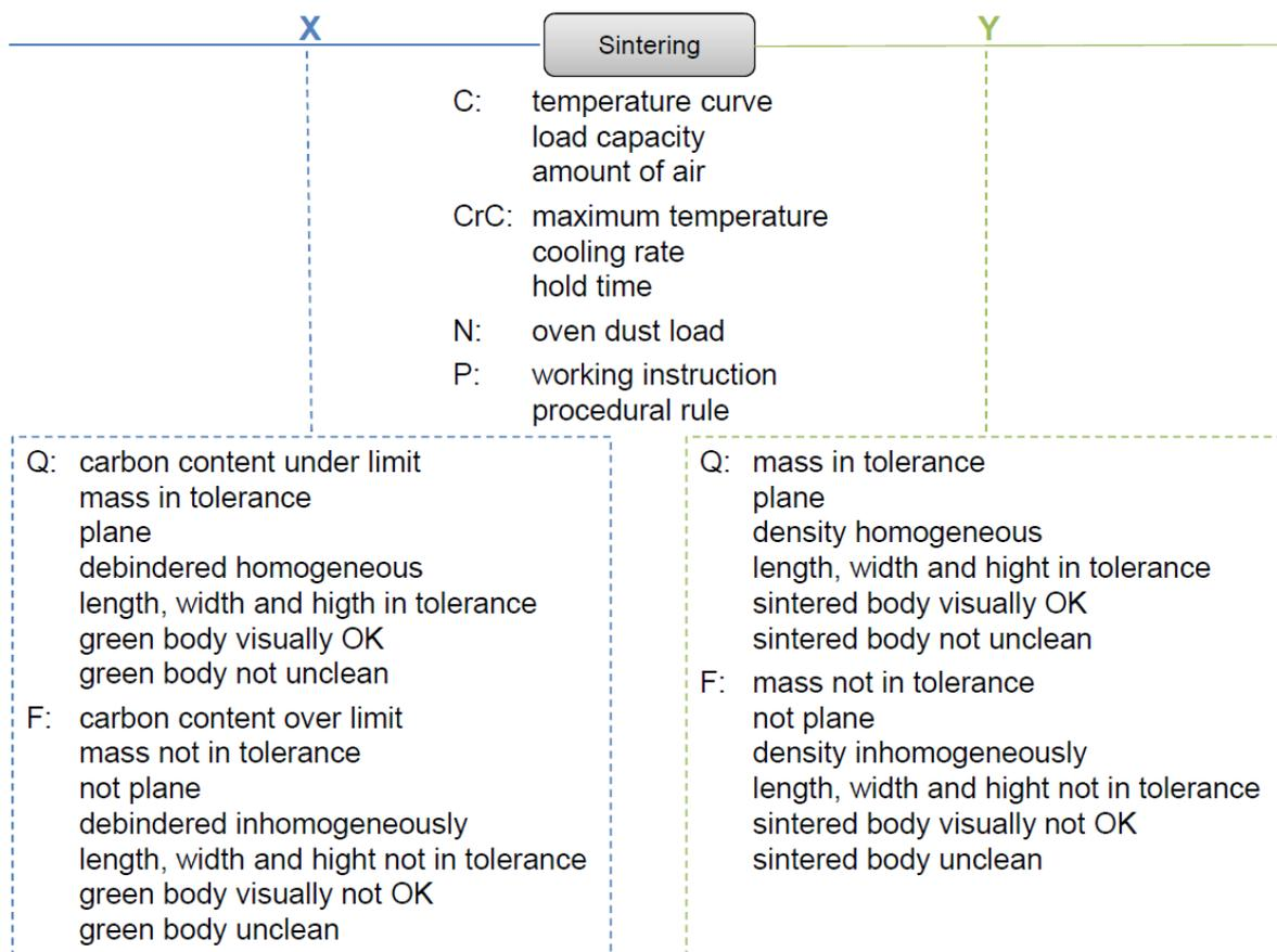
Figure 62: Process Mapping
