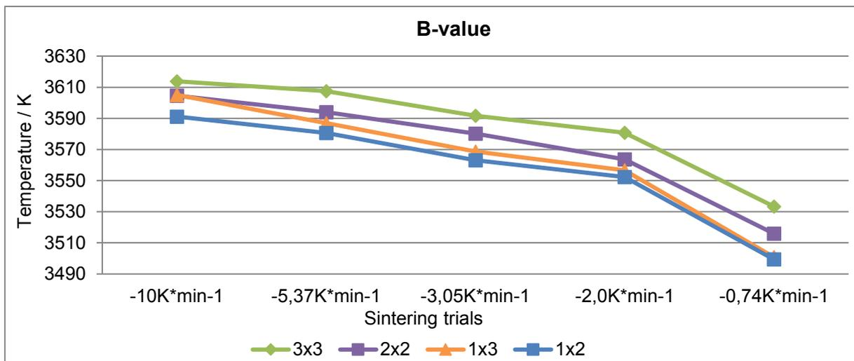
Figure 67: Evaluation of B-value with different cooling rates
