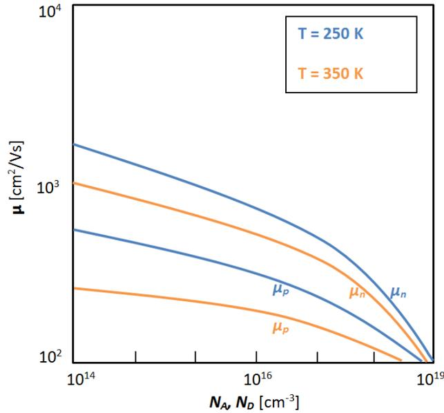
Figure 9: The mobility of electrons ( $\mu_n$ ) and holes ( $\mu_p$ ) for two different temperatures in a doped semiconductor.
