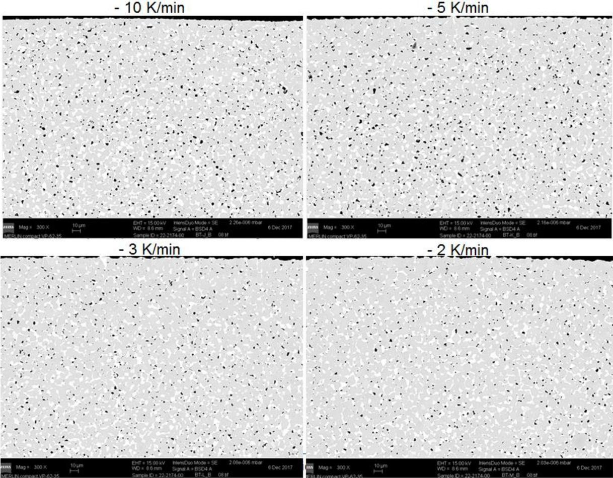
Figure 72: SEM pictures in BSE mode for the length of four different cooling rates
