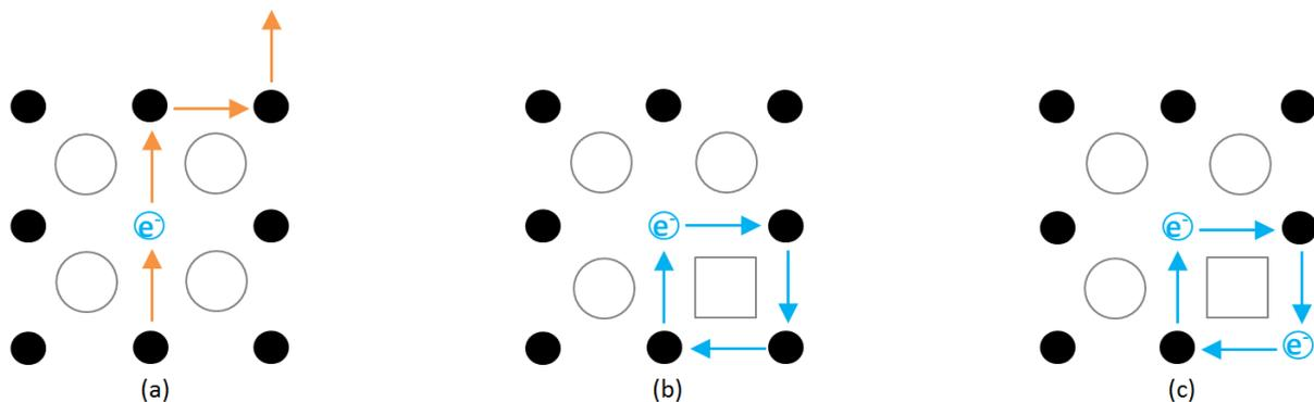
Figure 12: Schematic layout for the movement of polarons (a) free movement on lattice sites; (b) and (c) localized movement around lattice defects.
