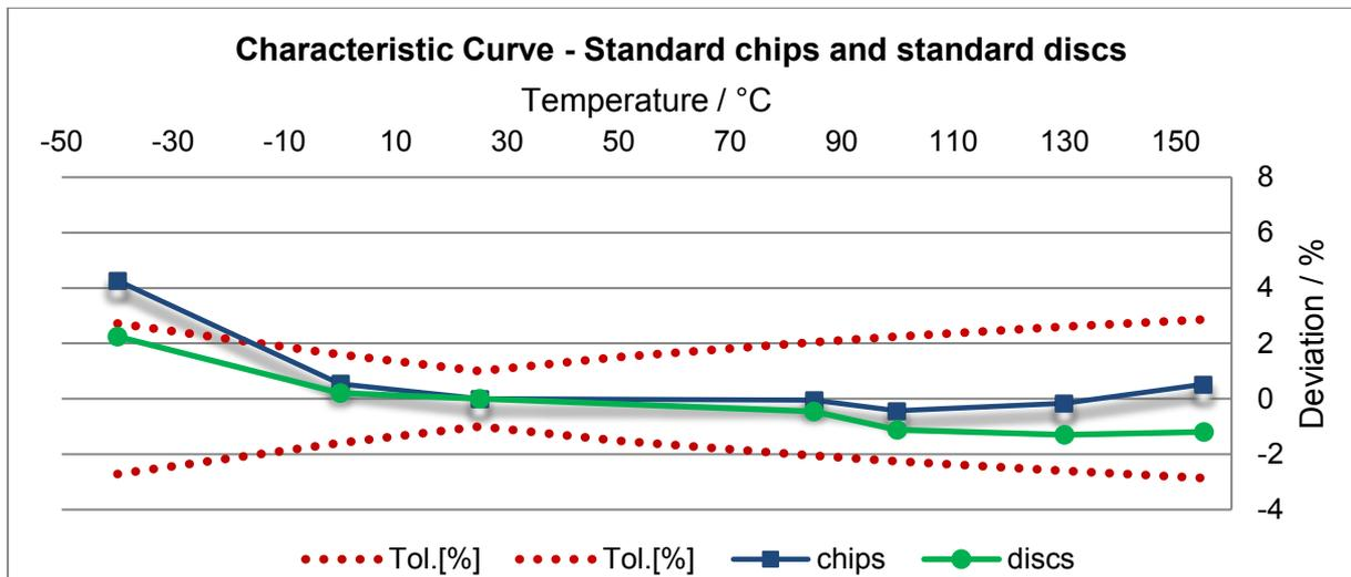
Figure 49: Characteristic curves of NTC standard chips and standard discs
