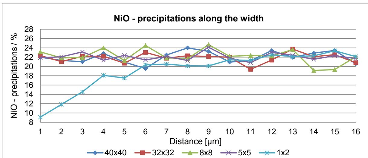
Figure 60: Precipitation distribution along the width from 1x2 mm<sup>2</sup> chips cut out from: 40x40, 32x32, 8x8 and 5x5 mm<sup>2</sup> substrates and 1x2 mm<sup>2</sup> non-standard chip
