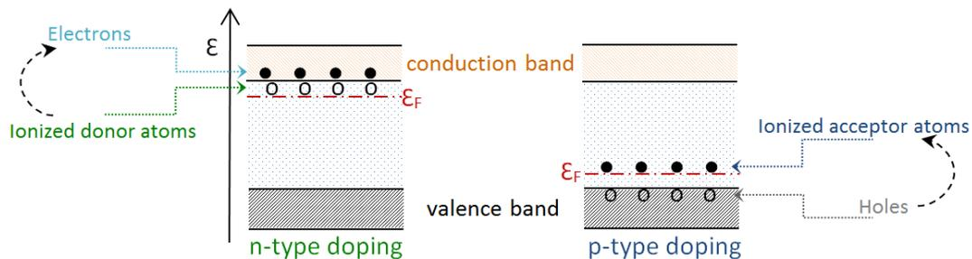
Figure 7: Band structure of doped semiconductors; on the left side occupation with electrons (●) of the conduction band at the bottom, on the right side occupation with holes (○) of the valence band at the upper edge.
