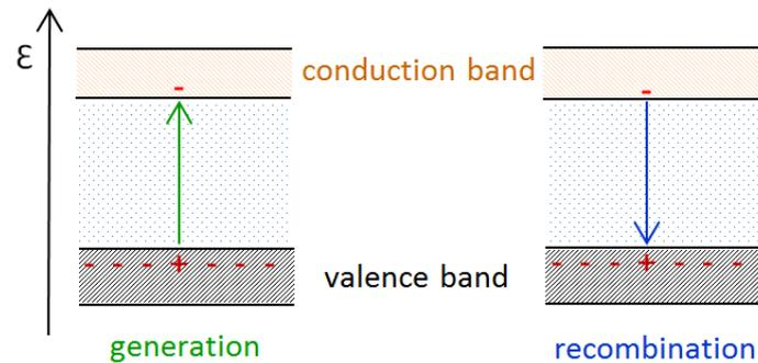
Figure 6: Band model of intrinsic semiconductor. Left side: generation of electron hole pair; Due to the removal of the electrons from the valence band holes are created. Right side: recombination of an electron with a hole.
