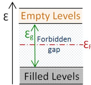
Figure 5: Band structure of semiconductor
