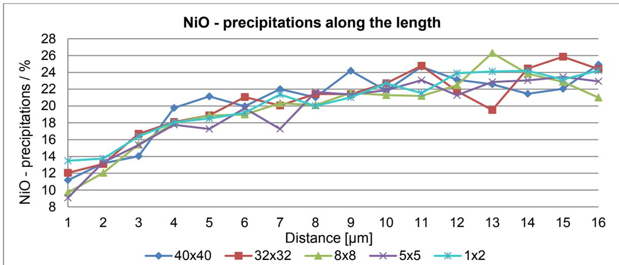
Figure 58: Precipitation distribution along the length from 1x2 mm<sup>2</sup> chips cut out of: 40x40, 32x32, 8x8, 5x5 mm<sup>2</sup> substrates and 1x2 mm<sup>2</sup> non-standard chips
