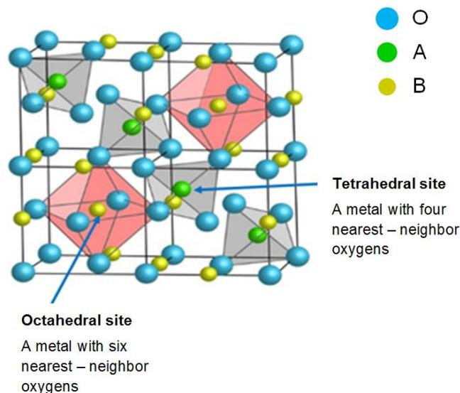
Figure 13: Half of the crystal structure of the normal spinel ( $AB_2O_4$ ) indicating the tetrahedral and octahedral sites. [38]
