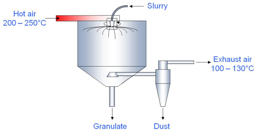
Figure 17: Spray dryer for spraying slurry into a warm drying medium (training material which has been kindly provided by TDK)
