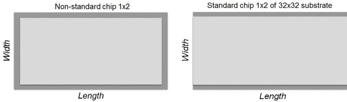
Figure 61: Comparison of NiO precipitation non-standard 1x2 mm<sup>2</sup> chip and standard chip 1x2 mm<sup>2</sup> chip cut out of a larger substrate after sintering. The region of higher amount of NiO precipitations is shaded light grey and the region of lower amount of NiO precipitations is shaded dark grey.
