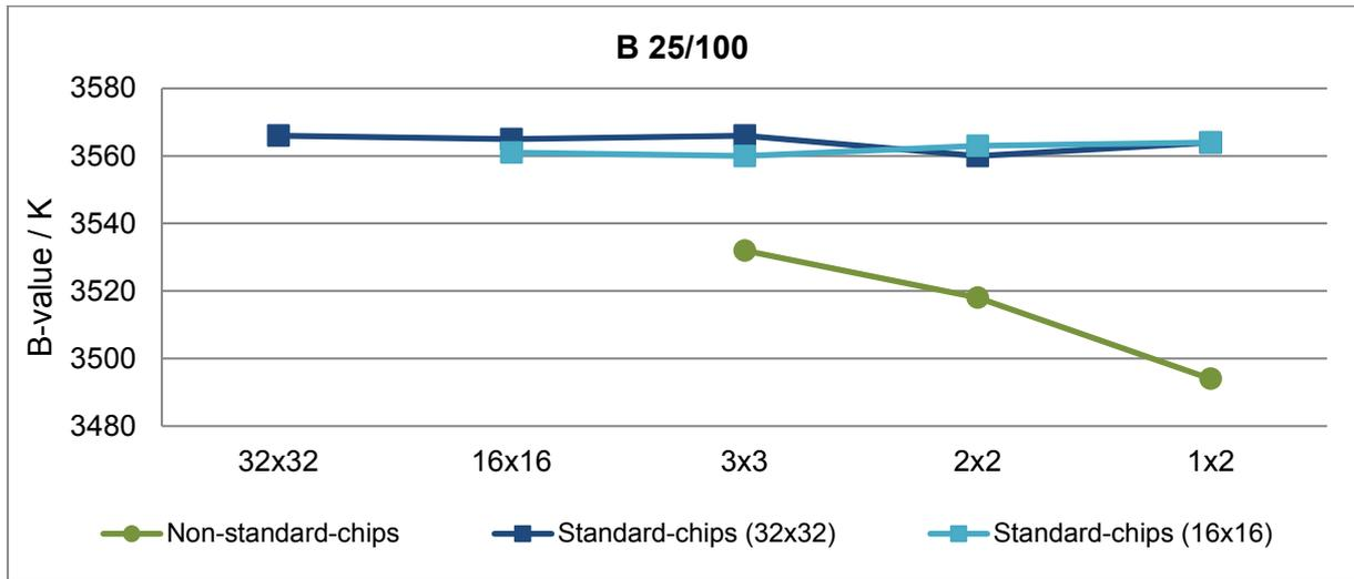
Figure 52: B-value of standard chips: 32x32 mm<sup>2</sup> (16x16, 3x3, 2x2 and 1x2) and 16x16 mm<sup>2</sup> (3x3, 2x2, and 1x2) and non-standard chips: 3x3, 2x2, and 1x2 mm<sup>2</sup>
