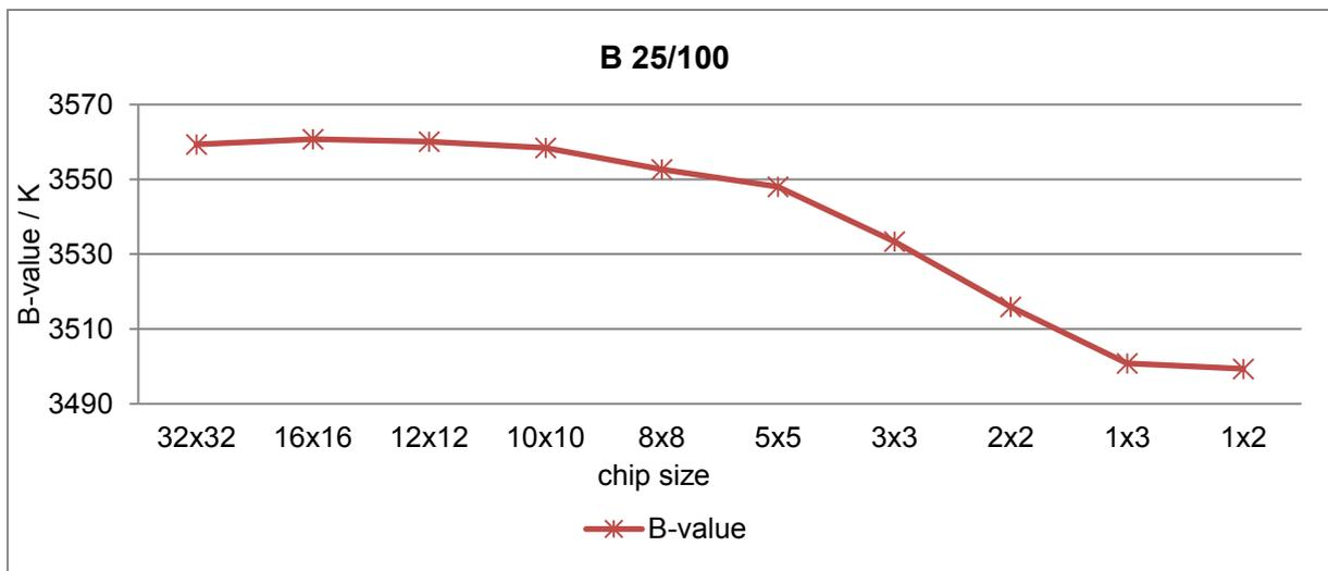
Figure 53: B-value of standard chips: 32x32 mm<sup>2</sup>, 16x16 mm<sup>2</sup> and non-standard chips: 12x12, 8x8, 5x5, 3x3, 2x2, 1x3 and 1x2 mm<sup>2</sup>
