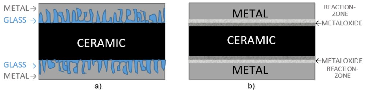
Figure 20: Schema of frit-bond type (a) and chemical-bond type (b)
