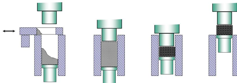
Figure 18: Steps of an axial compression (from left to right): Filling, prepressing, pressing and ejection motion (training material which has been kindly provided by TDK)
