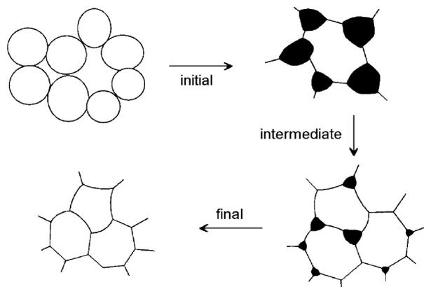
Figure 19: Microstructural changes during sintering [43]
