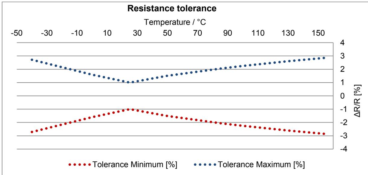
Figure 45: Characteristic curve with tolerance band
