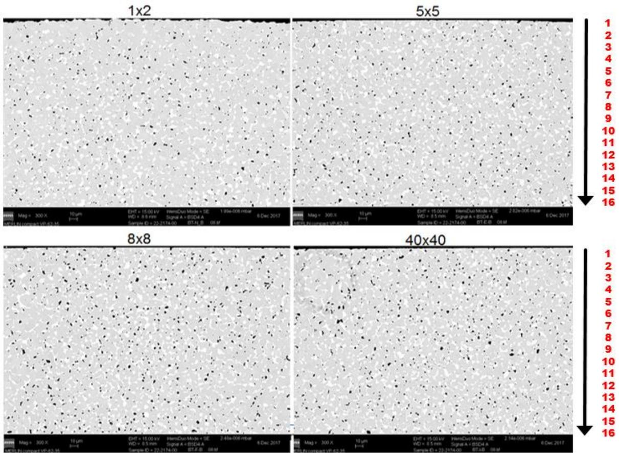
Figure 57: SEM pictures in BSE mode for the length in four different sinter geometries from 1x2 mm<sup>2</sup> chips cut out off: 40x40, 8x8 and 5x5 mm<sup>2</sup> substrates and 1x2 mm<sup>2</sup> non-standard chip
