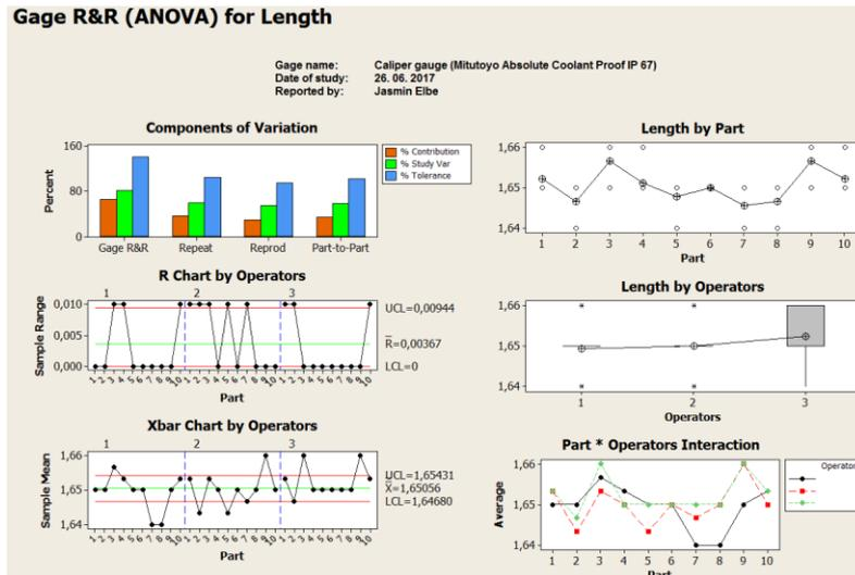
Figure 32: Graphical summary of the Gage R&R for the caliper gauge for the length
