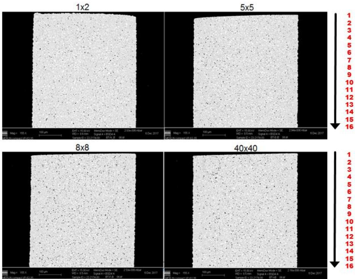
Figure 59: SEM pictures in BSE mode for the width in four different sinter geometries: from 1x2 mm<sup>2</sup> chips cut out from: 40x40, 8x8 and 5x5 mm<sup>2</sup> substrates and 1x2 mm<sup>2</sup> non-standard chip
