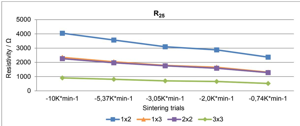
Figure 68: Evaluation of  $R_{25}$  with different cooling rates
