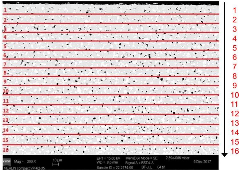
Figure 43: Example for a picture with BSE for the determination of NiO precipitation
