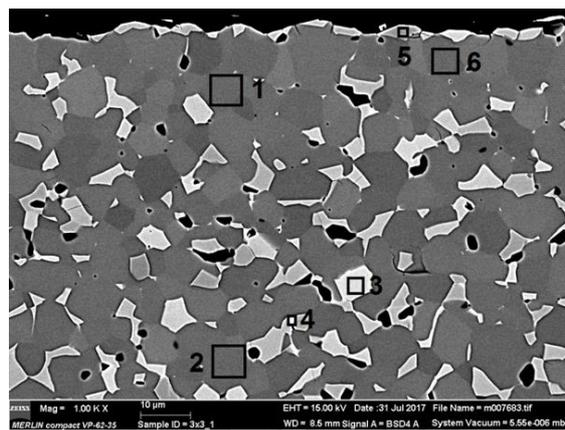
Figure 56: Microstructure of ceramics with EDX analysis (area indicated by numbered square).
