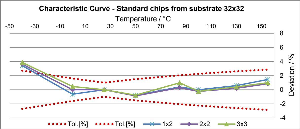
Figure 47: Characteristic curves of standard chips:  $1\times 2$ ,  $2\times 2$ ,  $3\times 3\text{ mm}^2$  cut from standard substrate  $32\times 32\text{ mm}^2$
