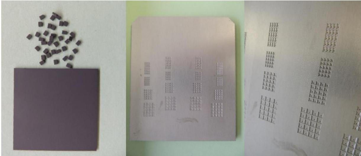
Figure 26: Cut substrates in the size of 32x32 mm<sup>2</sup> compared with 2x2 mm<sup>2</sup> chips on the left side - special metallization device in the middle and on the right side for metallization of 3x3, 2x2, 1x3 and 1x2 mm<sup>2</sup> non-standard chips
