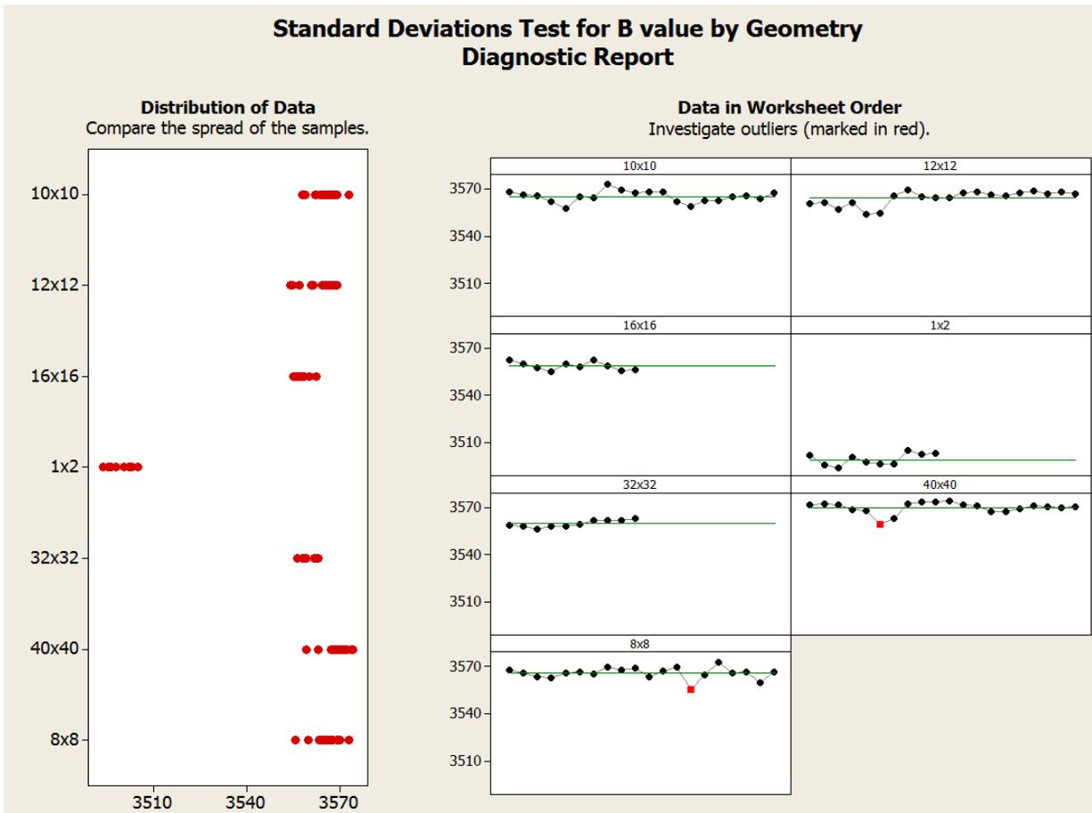
Figure 55: Standard deviation test for B-value by geometry of 1x2 standard substrates: 32x32 mm<sup>2</sup> and 16x16 mm<sup>2</sup> and non-standard substrates: 40x40, 12x12, 10x10, 8x8 mm<sup>2</sup> and the non-standard chip 1x2 mm<sup>2</sup> (without cutting).
