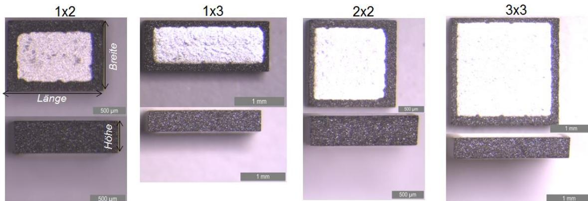
Figure 25: Metallized NTC non-standard chips in four different sizes: 3x3, 2x2, 1x3, 1x2 mm<sup>2</sup>
