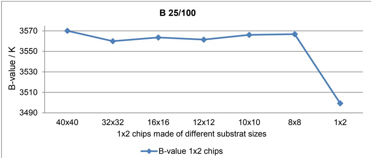
Figure 54: B-value of 1x2 mm<sup>2</sup> chips of standard substrates: 32x32 mm<sup>2</sup> and 16x16 mm<sup>2</sup> and non-standard substrates: 40x40, 12x12, 10x10, 8x8 mm<sup>2</sup> and the non-standard chip 1x2 mm<sup>2</sup> (without cutting).
