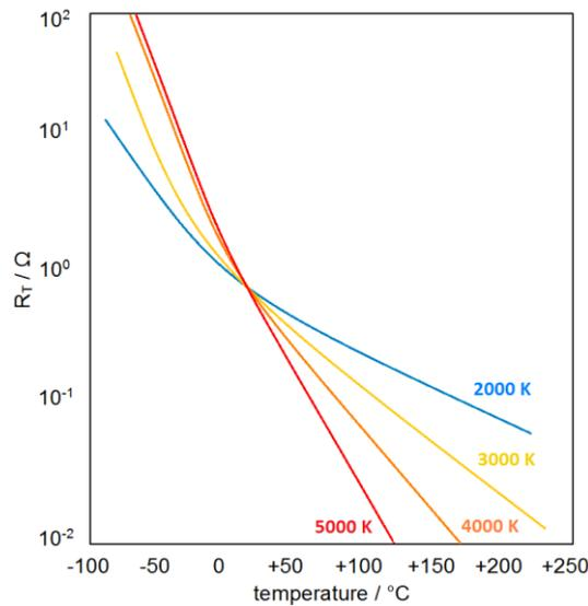
Figure 4:  $R_T$  of NTC - thermistors based on  $R_{25}$  from four different B-values as a function of temperature [11]
