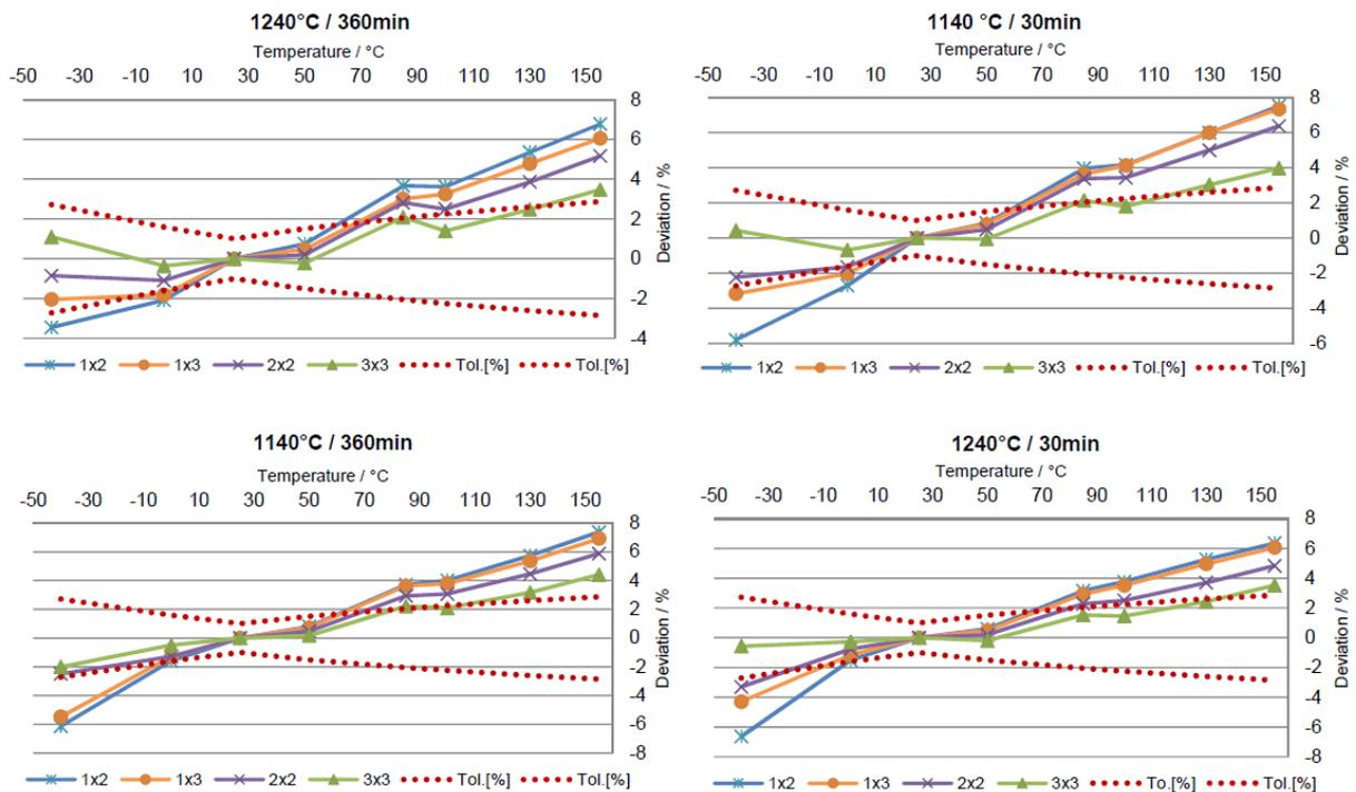
Figure 65: Evaluation characteristic curves Sinter DoE (cooling rate 0,74 K/min)
