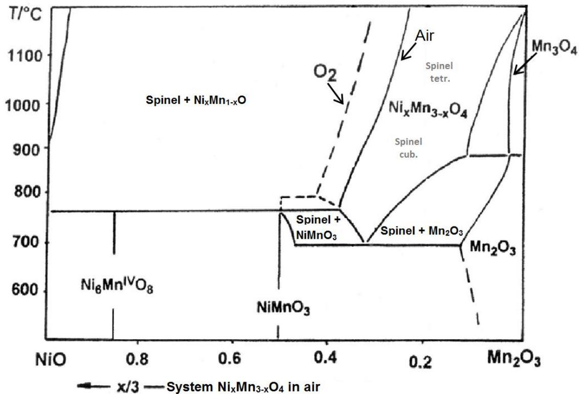
Figure 15: Phase diagram for the system Ni-Mn-O, adapted from Wickham [40]
