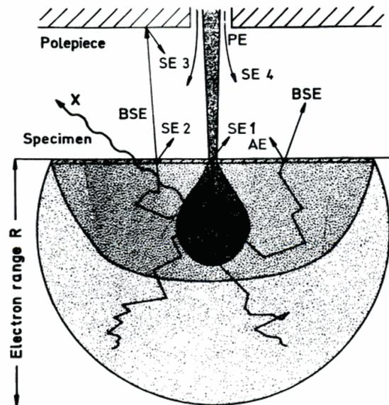
Figure 42: Scanning electron microscope – interaction volume
