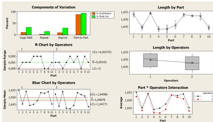
Figure 38: Graphical summary of the Gage R&R for the micrometer calliper
