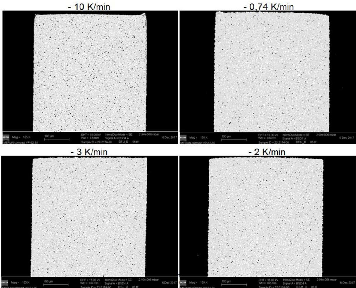
Figure 74: SEM pictures in BSE mode for the width of four different cooling rates
