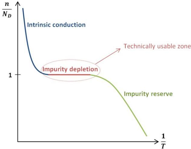
Figure 8: Correlation between the charge carrier concentration and the temperature in the valence band of an n-type semiconductor
