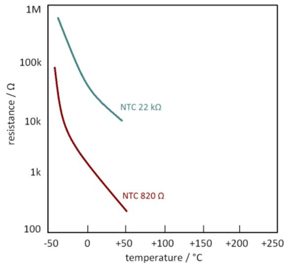
Figure 3: Characteristic curve of two types of NTC-resistors according to DIN 44070 [9]
