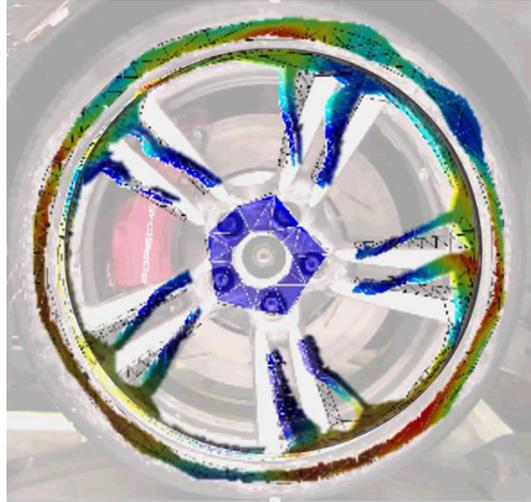
Figure 5.5: Laser-vibrometry measurements of rim deflections during brake moan, from [45]
