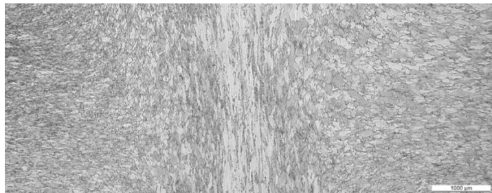
Figure 10: Cross-section rotary friction welded (RFW) commercially pure molybdenum with PWHT [68]
