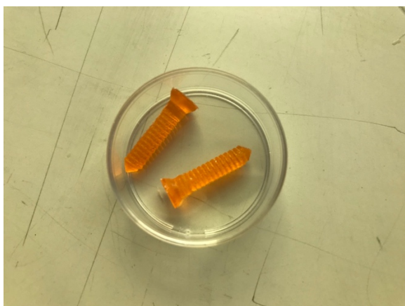
Figure 28 3D printed bone screws from a ternary system containing DBC.
