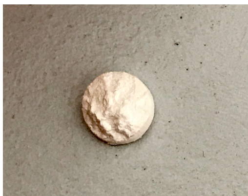
Figure 31 Test 3D-print of a bone screw consisting of a ternary system filled with Al 2 O 3 .
