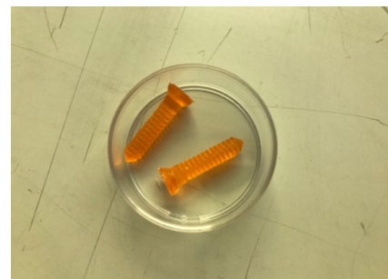
Figure 38 3D printed bone screws with a ternary system containing DBC.
